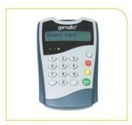
Perfect for corporate, administrative, eCommerce and eBanking services that require an extra layer of security, the PC Pinpad integrates a tactile 16 key keypad, a 2x16 line display and a USB interface.
