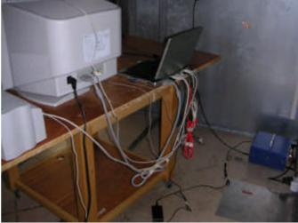
The EST and auxiliaries are set on the no-conductive table of 80 cm height. The AC-DC power supply is set on the floor.
