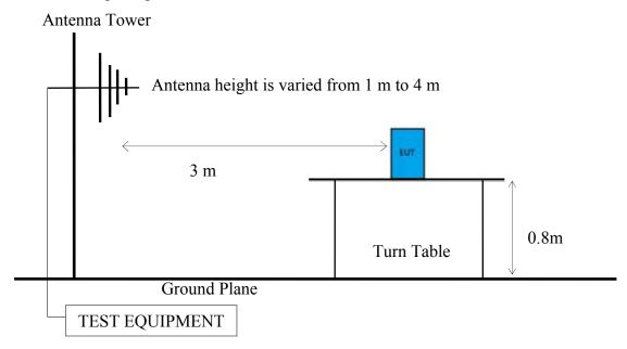
6.1.3. Semi-Anechoic Chamber (3m) Setup Diagram for above 1GHz
