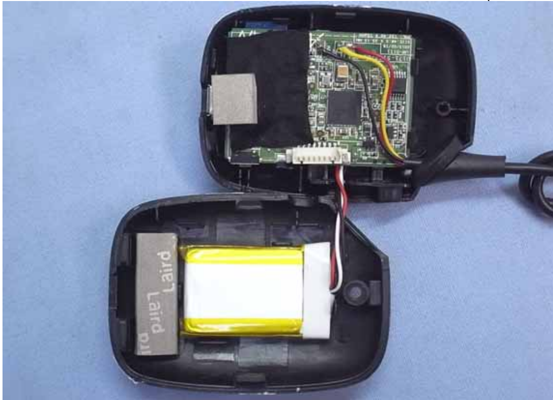
Figure 12 Internal View (Battery)
