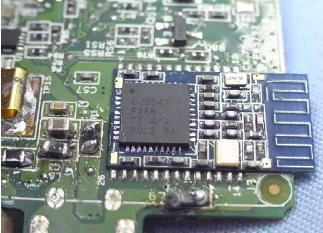
Figure 15 Internal View (BLE Module, Front View)
