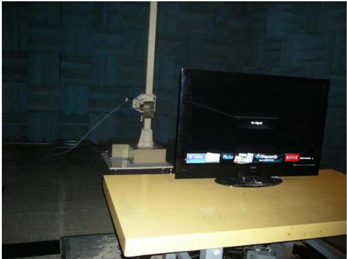
FRONT VIEW OF RADIATED MEASUREMENT
