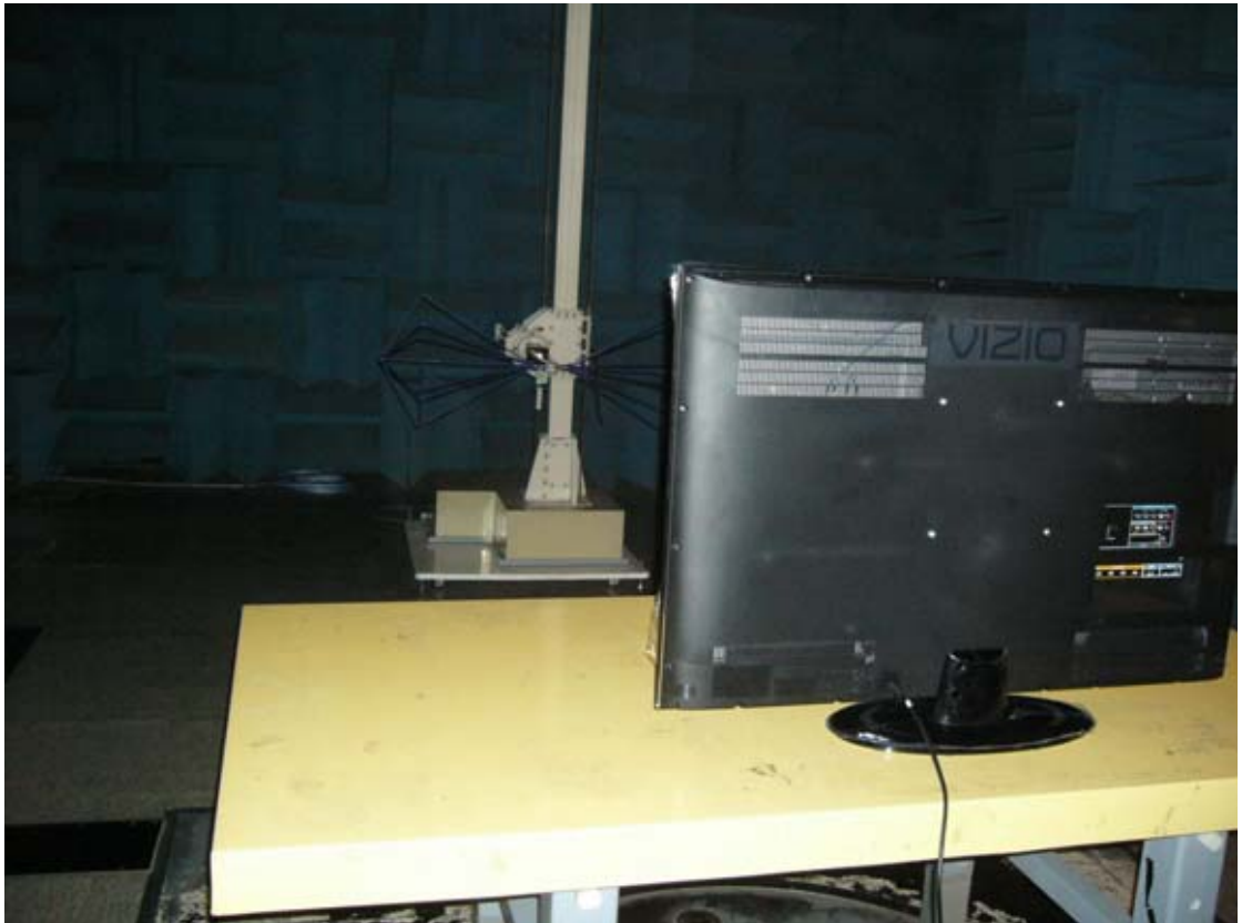
BACK VIEW OF RADIATED MEASUREMENT
