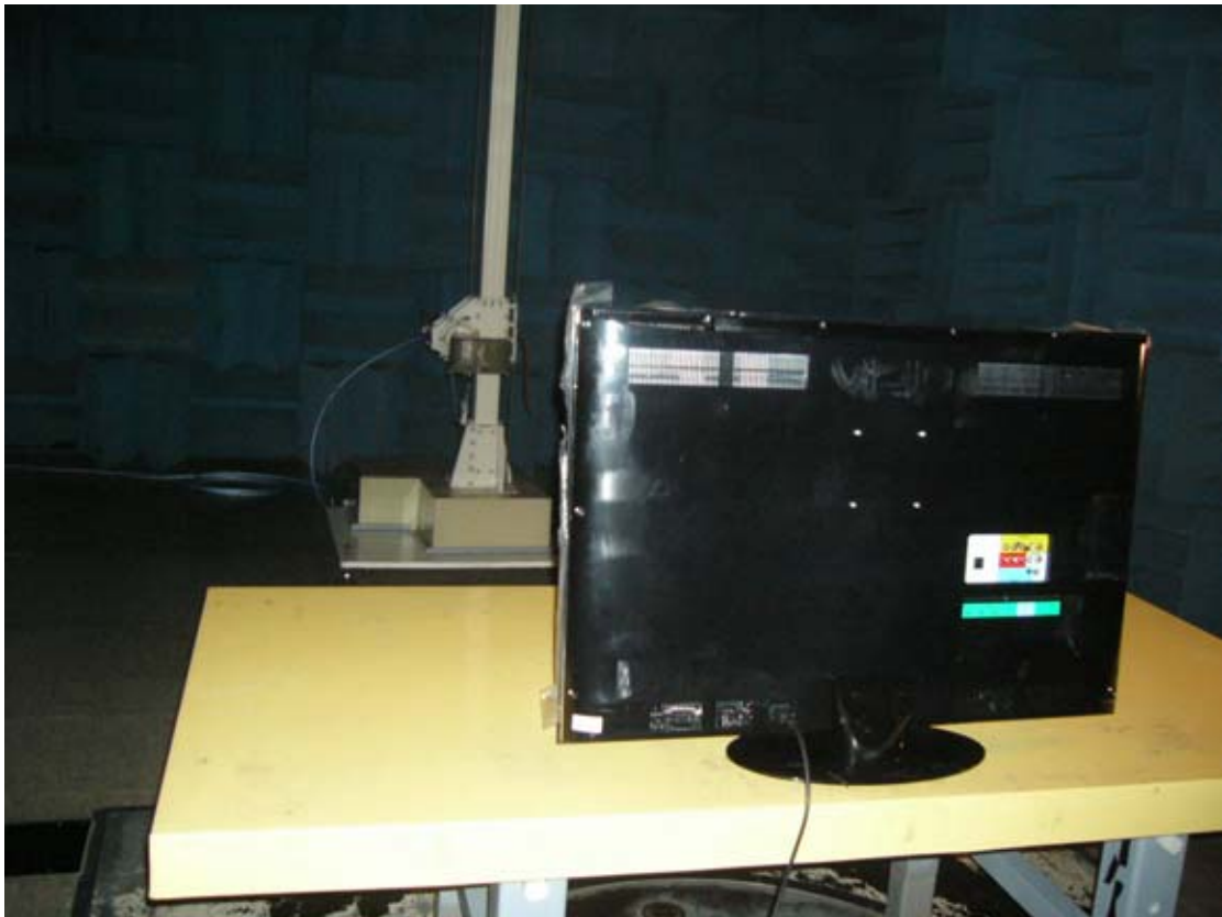
BACK VIEW OF RADIATED MEASUREMENT
