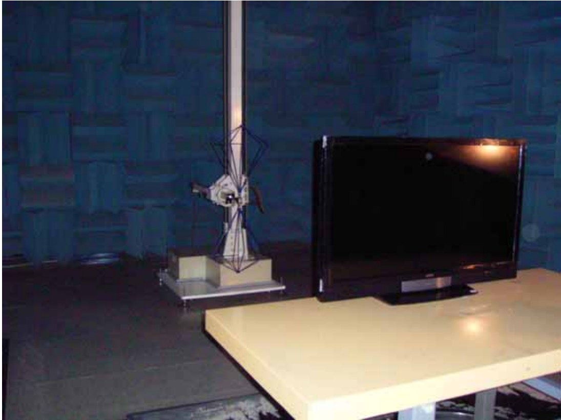
FRONT VIEW OF RADIATED MEASUREMENT
