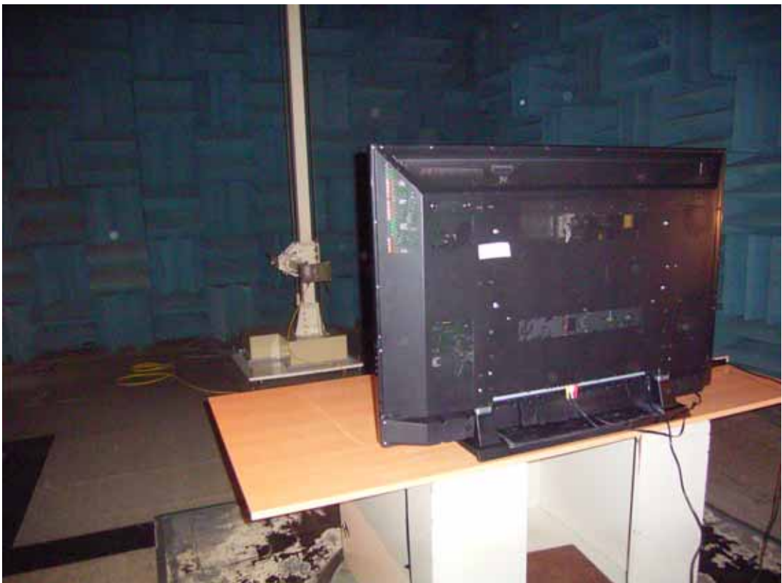
BACK VIEW OF RADIATED MEASUREMENT
