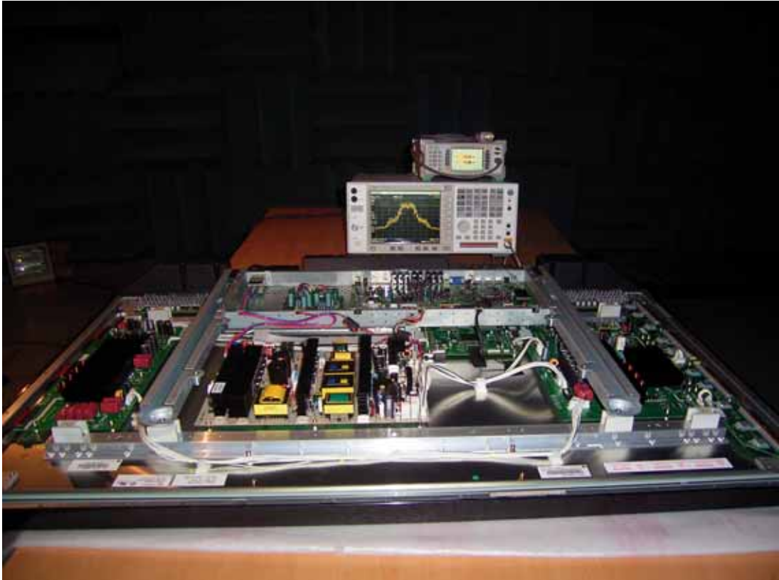
10.3.Photo of 6dB Bandwidth Measurement (Conducted)
