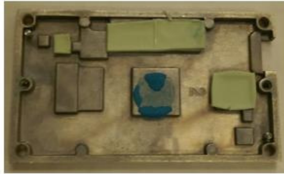
Heat Sink Internal View
