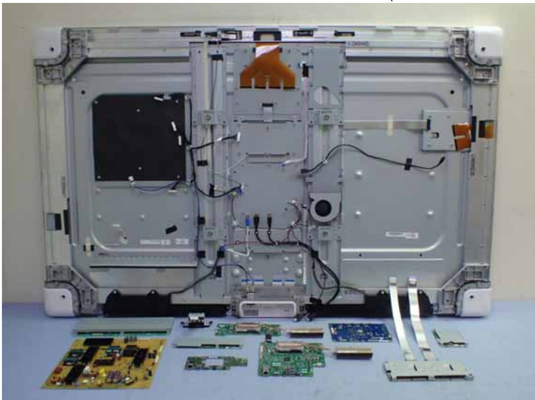
Figure 8 Internal View (Removed Internal Boards)
