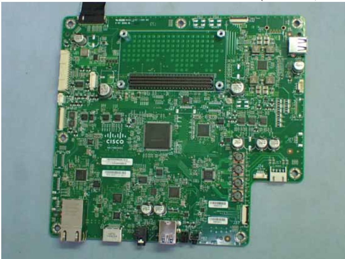
Figure 24 Internal View (Main Board, Front View)
