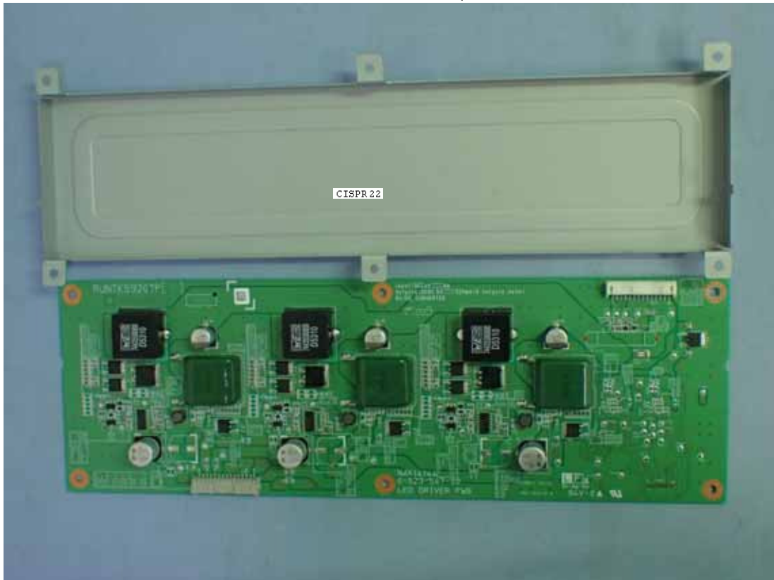
Internal View (DC/DC Converter Board, Front View)
