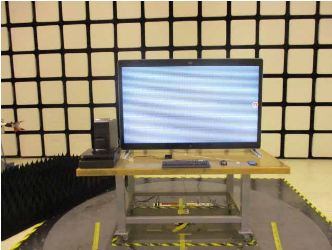
Front View of Radiated Measurement
