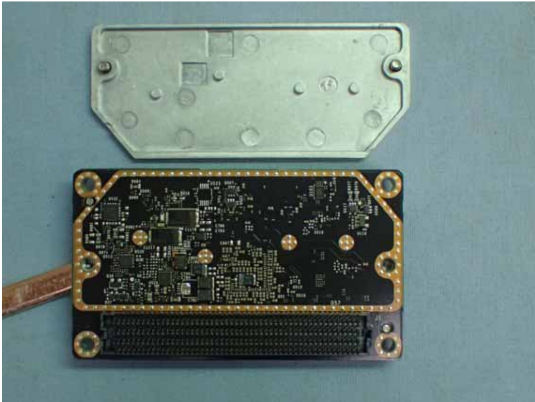
Figure 27 Internal View (RF Module, Back View)
