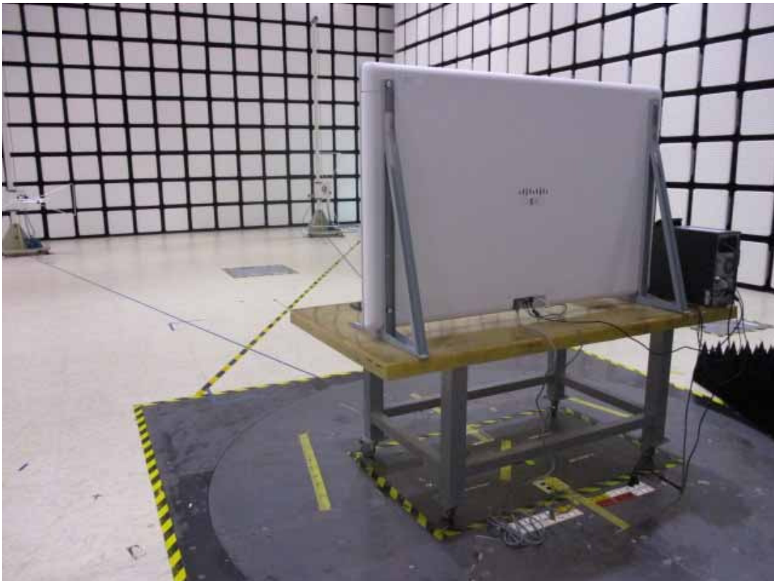
Back View of Radiated Measurement
