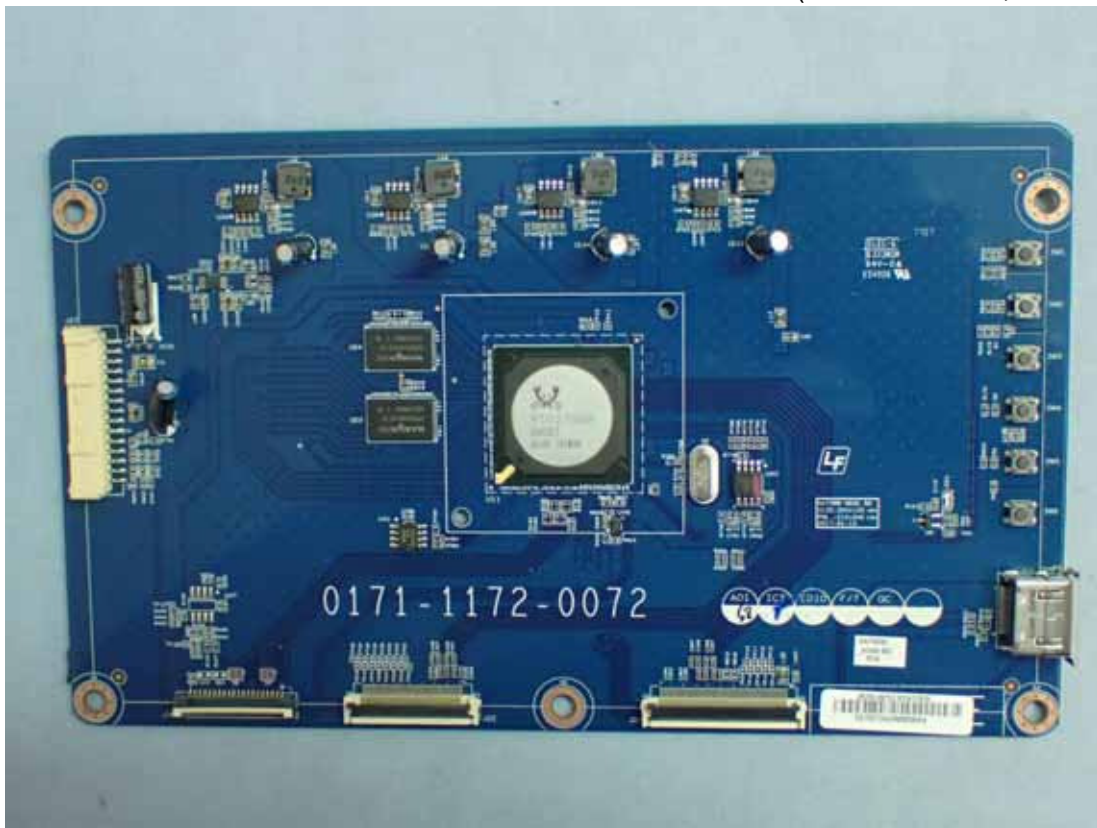
Figure 17 Internal View (Control Board, Front View)
