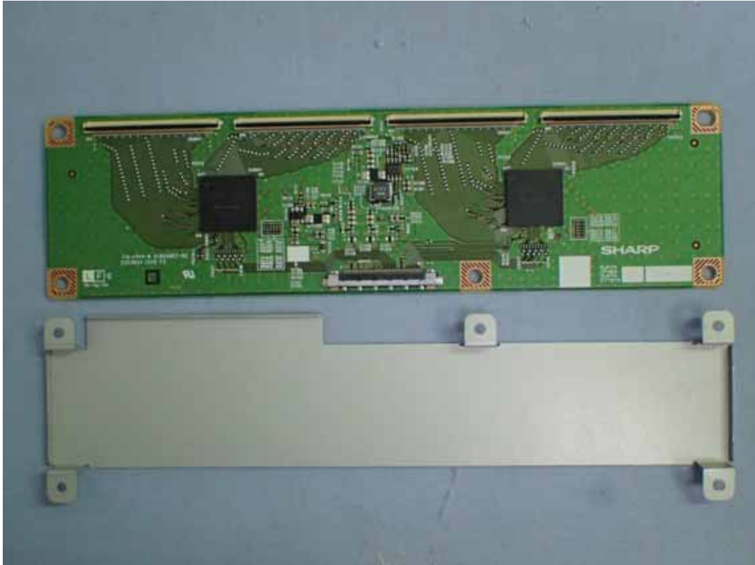
Internal View (Control Board, Front View)
