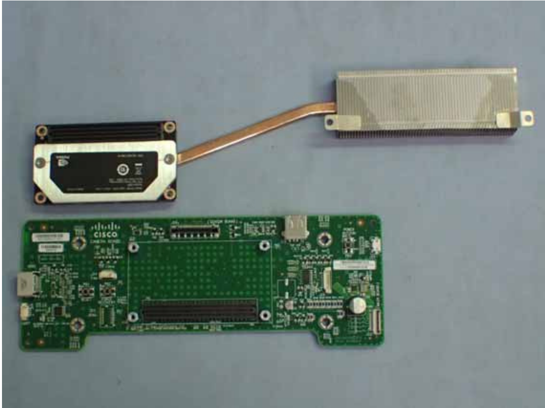
Figure 20 Internal View (Control Board, Front View)
