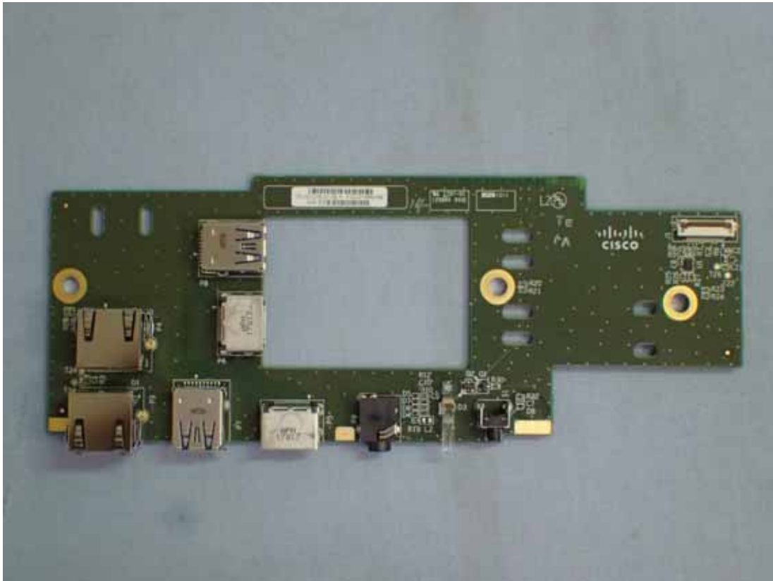
Figure 15 Internal View (I/O Ports Board, Front View)
