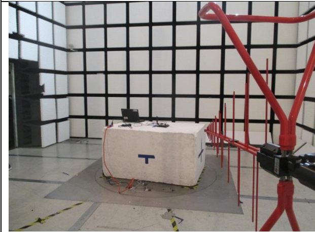
RADIATED FRONT PHOTO (BELOW 1 GHz)
