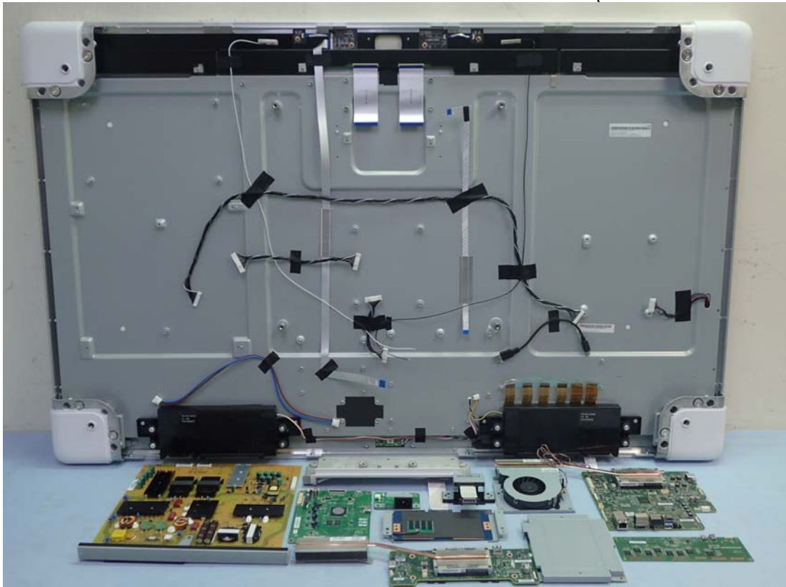
Figure 9 Internal View (Removed Internal Boards)
