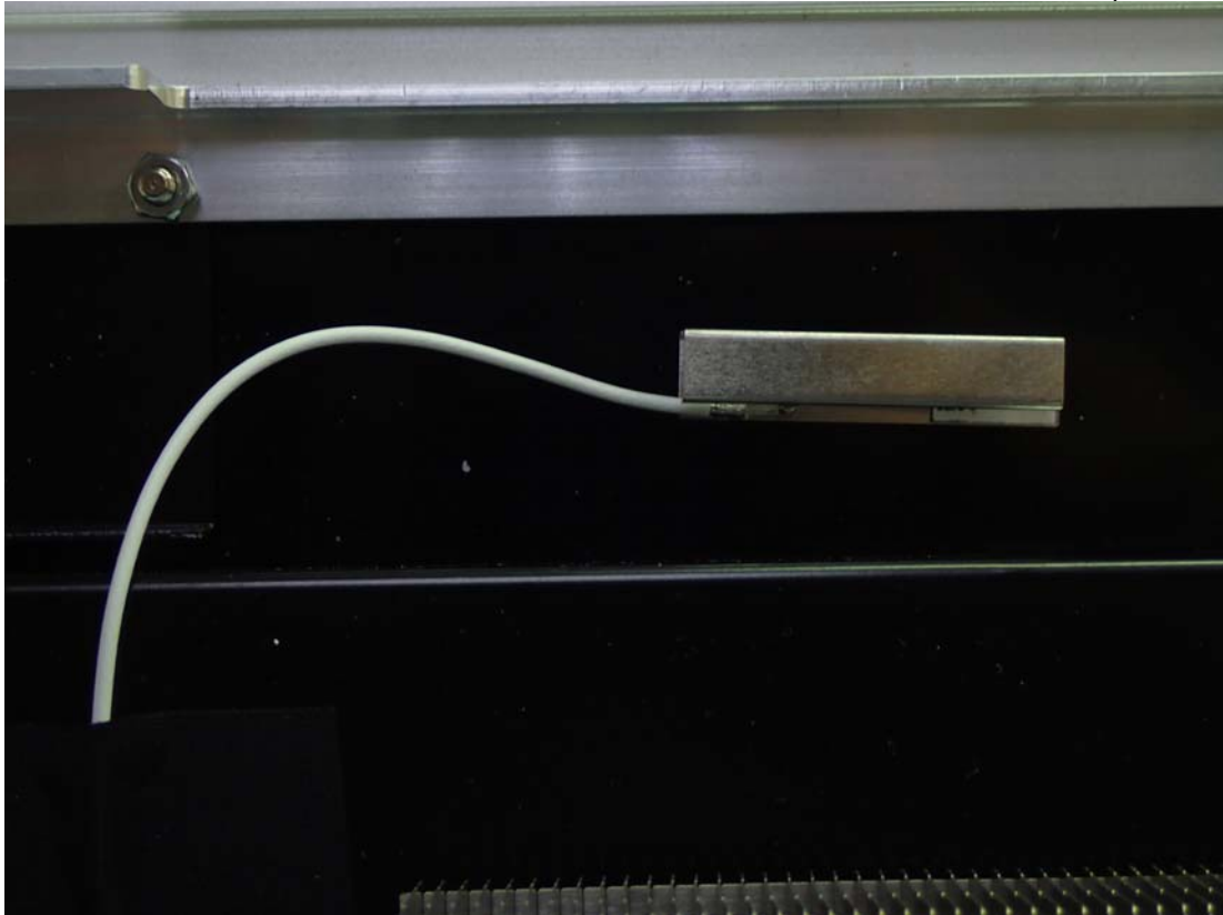
Figure 8 Internal View (Antenna View)
