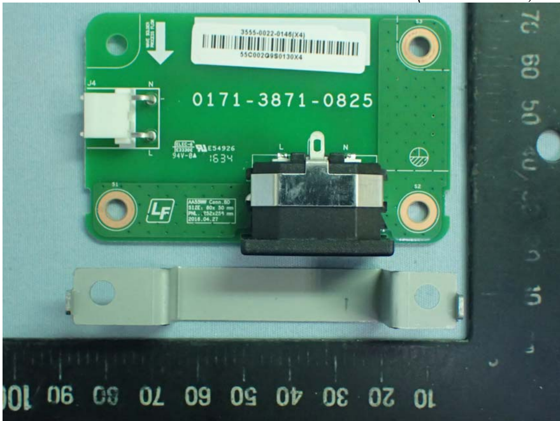
Figure 14 Internal View (AC Inlet Board, Front View)
