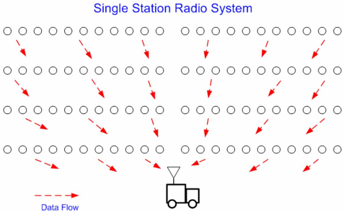
**All sensors have an independent communication path to the recording system**
