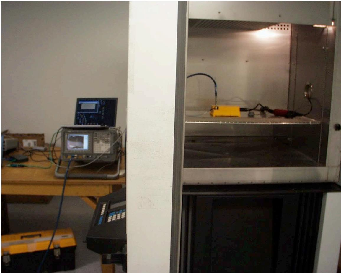
**Frequency Stability (Frequency v Operating Voltage)**
