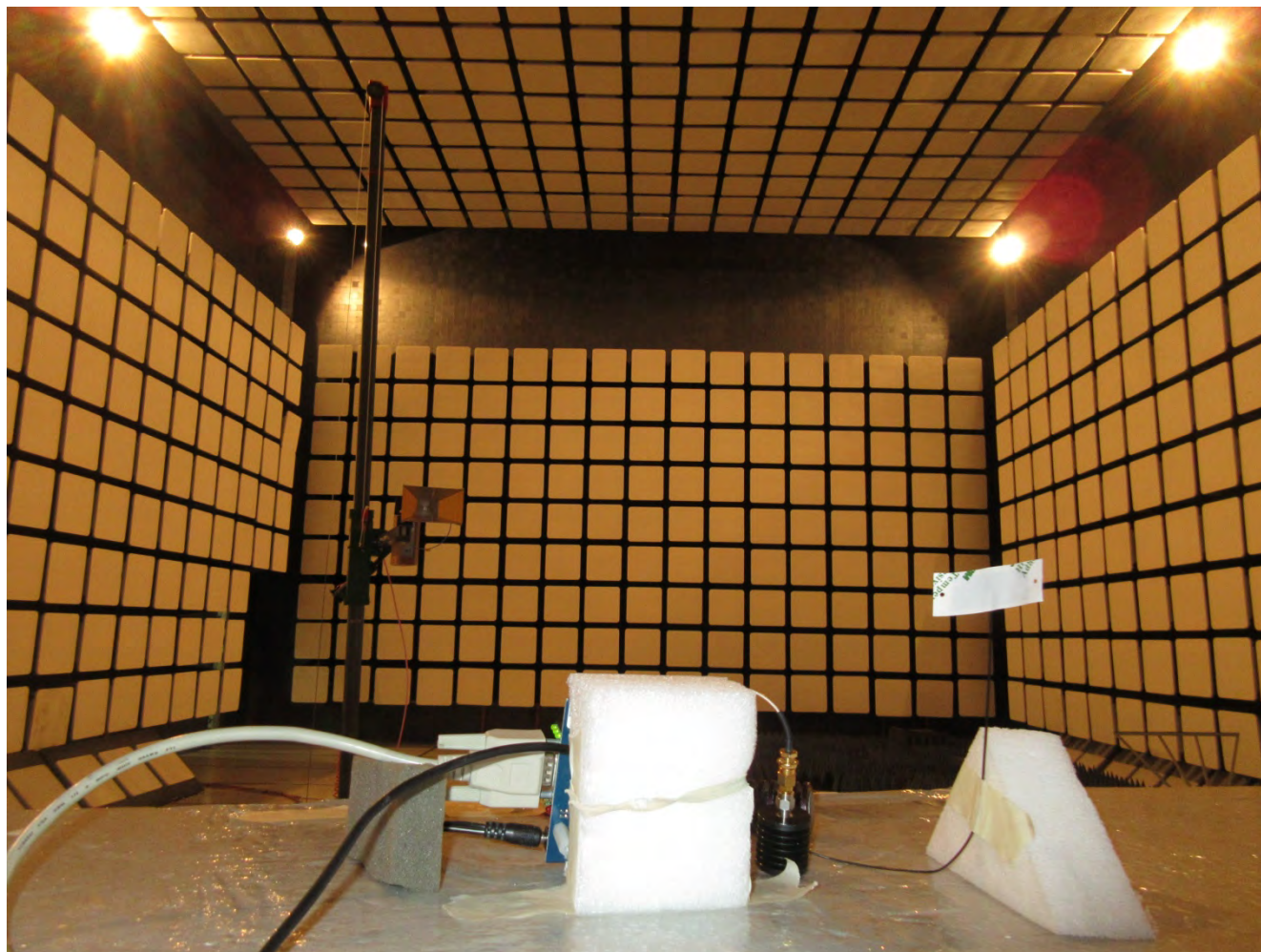
Radiated Emissions @ 3 m, Orthogonal Position 3
