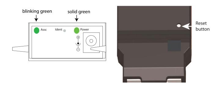
**Power LED**: Indicates that power is on. Illuminated only when adapter is connected to
