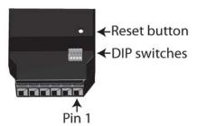
To insert or remove wires, insert a screwdriver blade in the slot directly below the hole where the wire inserts. Press down on the spring to open up the hole and insert or remove the wire.
