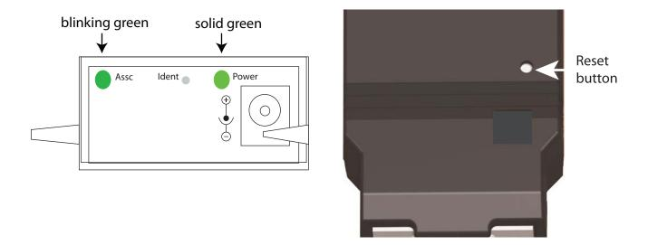
Indicates that power is on. Illuminated only when adapter is connected to external power only, not when powered by batteries. Not available in lithium-battery models. Power LED:
