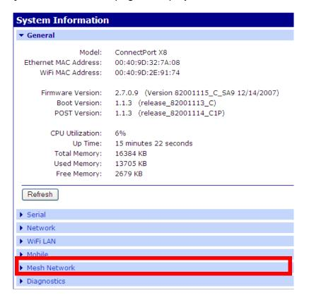
From the list of System Information links, click Mesh Network. The Mesh Network page is displayed. It shows several settings for the gateway, followed by the Network View of the Mesh Devices. In the Type column, the ZigBee module in the gateway is listed as the coordinator, and any XBee adapter/router/sensor products discovered are listed as routers.
