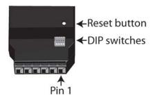
The adapter is switch-selectable between RS-422 half duplex, RS-422 full duplex, and RS-485 modes (see DIP switches, below). The function for several pins varies between RS-422 and RS-485 modes.
