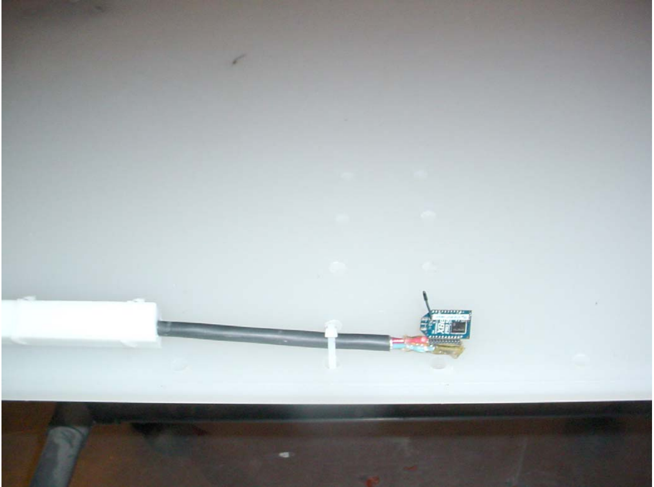
Radiated Emissions at 3 m EUT with 1.5 dBi Integrated Whip Monopole Antenna (Orthogonal Position 1)
