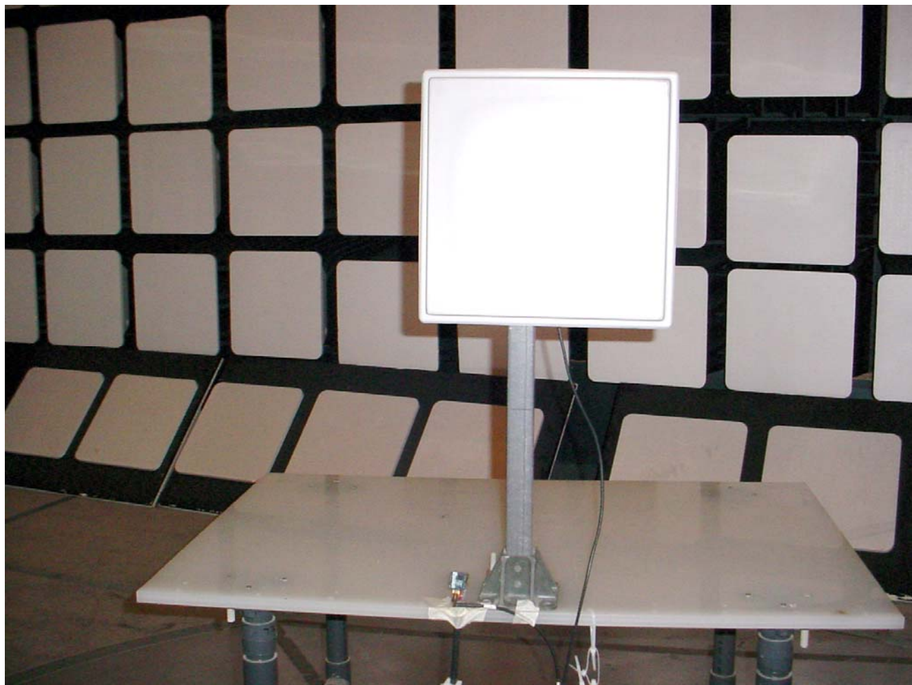
Radiated Emissions at 3 m EUT with 19 dBi Panel Antenna
