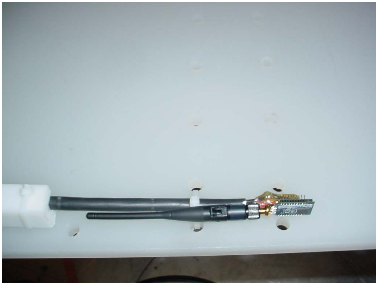
Radiated Emissions at 3 m EUT with 2.1 dBi Dipole Antenna in Horizontal Position
