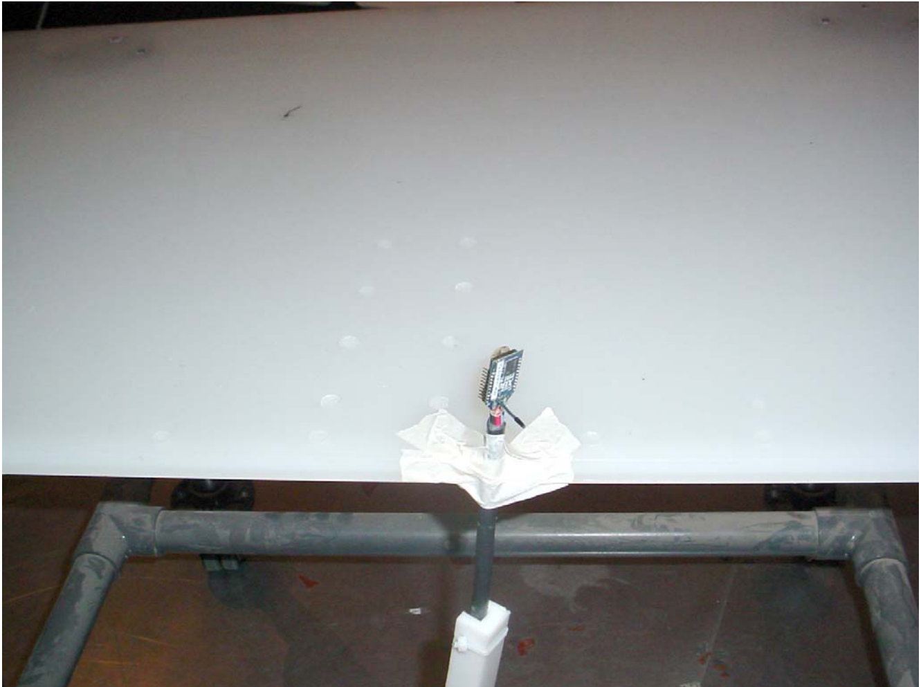
Radiated Emissions at 3 m EUT with 1.5 dBi Integrated Whip Monopole Antenna (Orthogonal Position 2)
