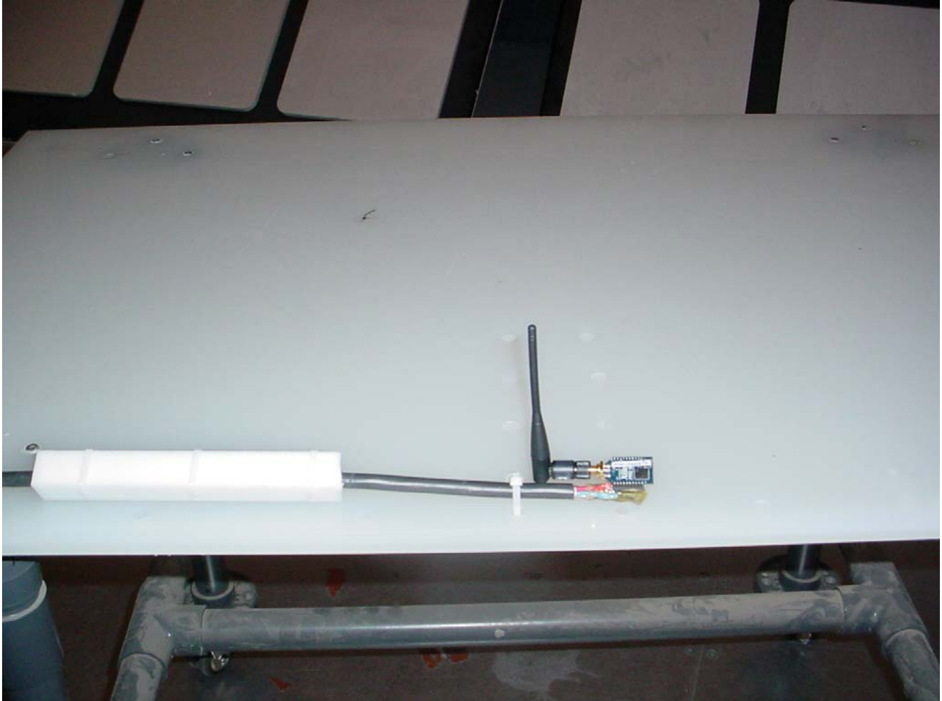
Radiated Emissions at 3 m EUT with 2.1 dBi Dipole Antenna in Vertical Position
