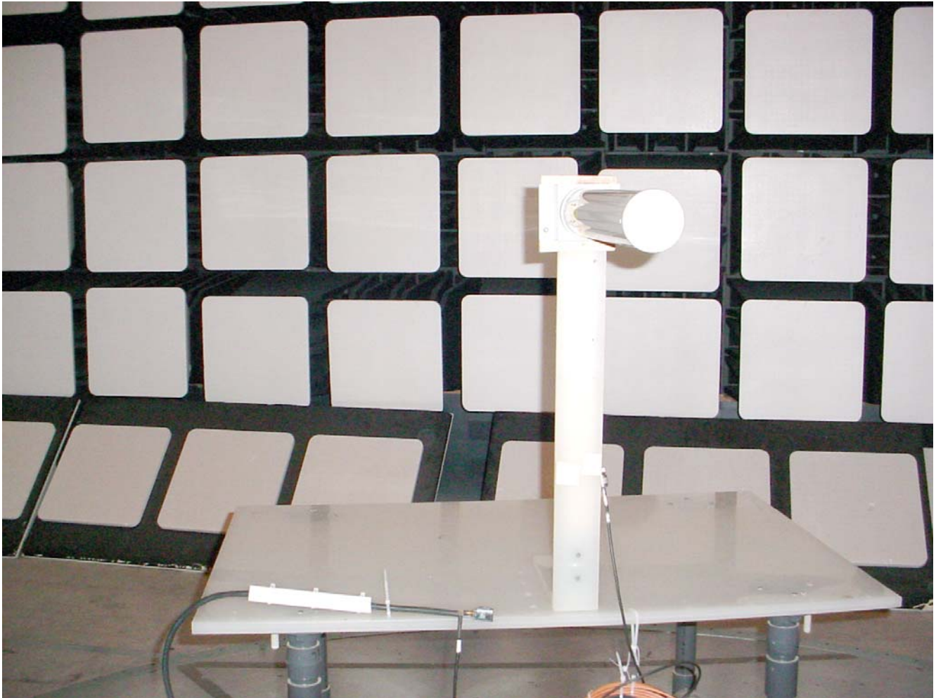
Radiated Emissions at 3 m EUT with 15 dBi Yagi Antenna
