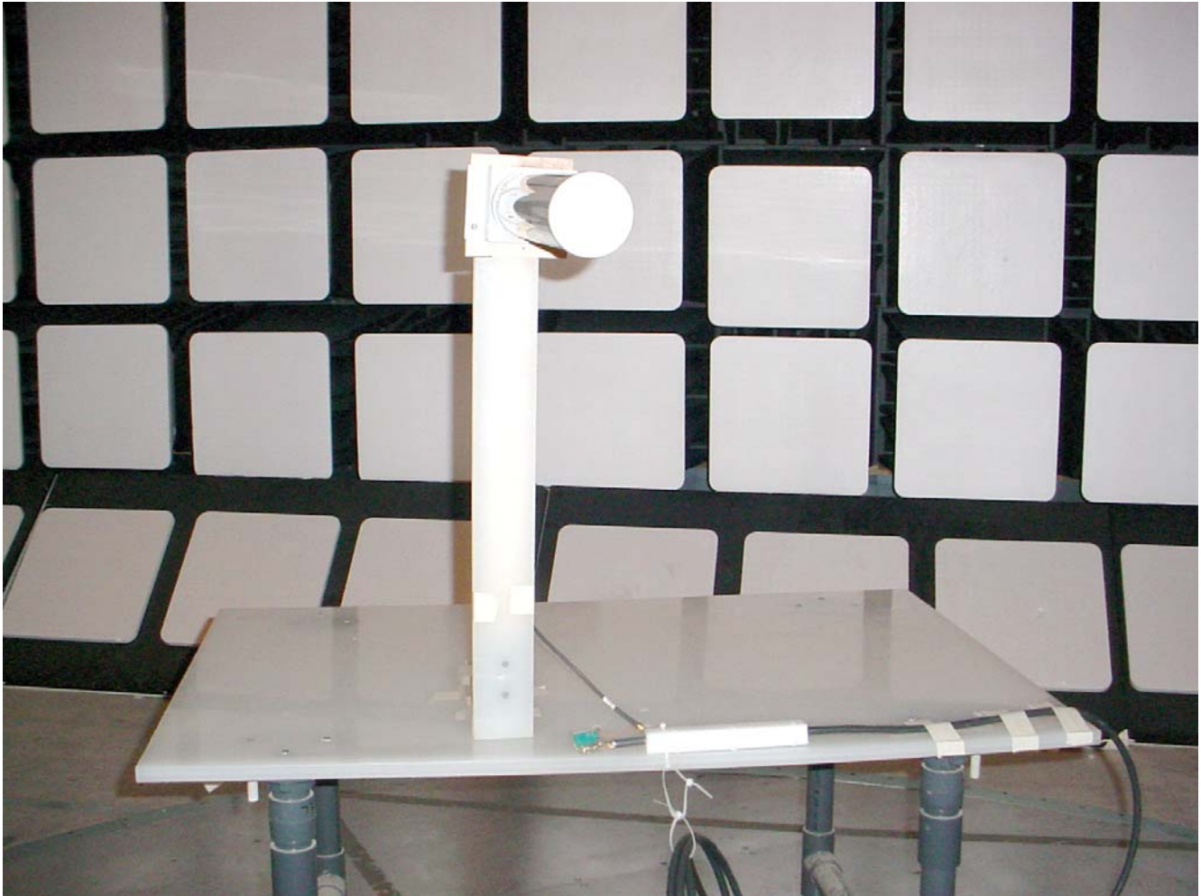
Radiated Emissions at 3 m EUT tested with Yagi Antenna (Max. Antenna Gain: 15 dBi)
