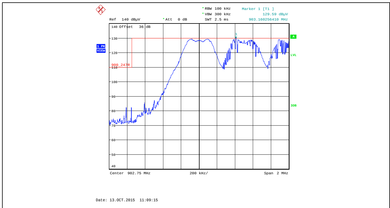
Plot 5.5.4.1.2.20. Band-Edge RF Radiated Emissions at 3 m, Vertical Polarization Pseudorandom Hopping Mode, Low End of Frequency Band, 902.75 MHz, XB2, Data Rate at 250 kbps
