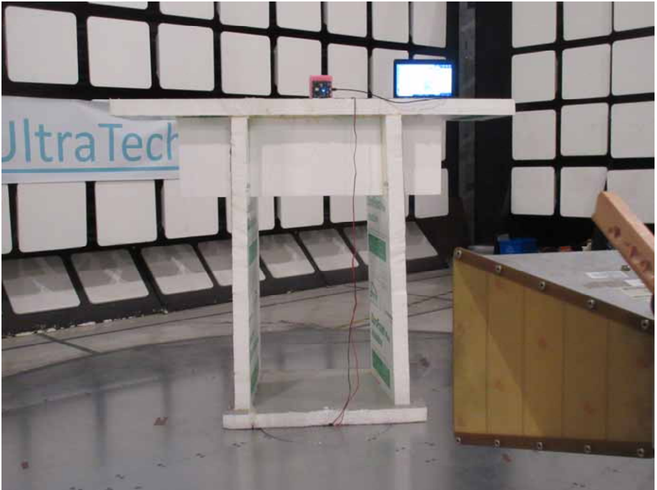
Radiated Emissions @ 3 m Orthogonal Position 2
