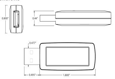
The following table provides the dimensions for the XBee 3 USB Adapter Pro.
