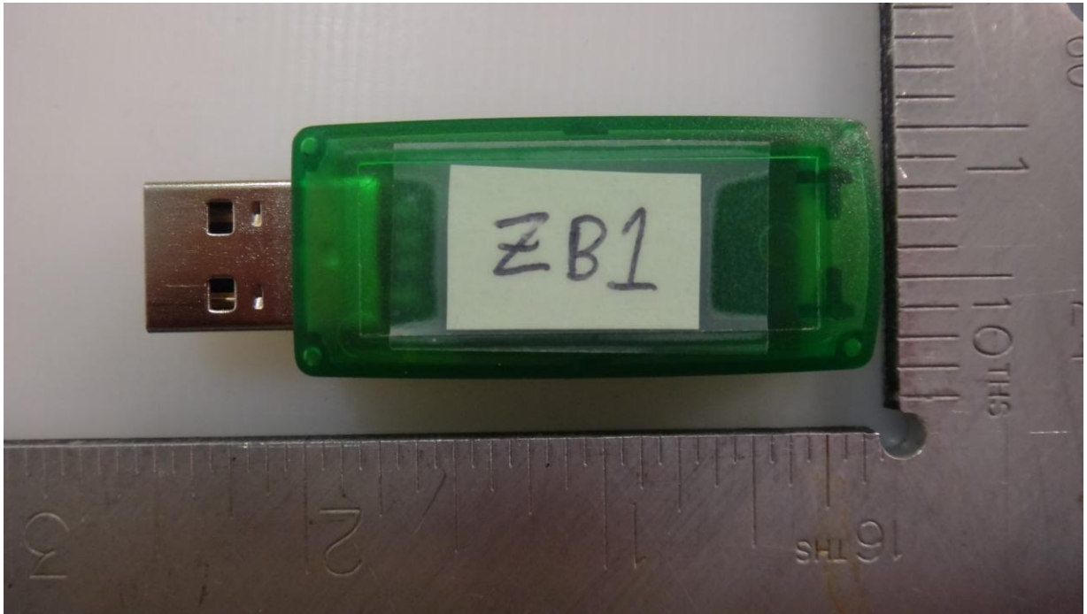
< D.U.T.'s front view with 802.15.4 Encoded Radio >
