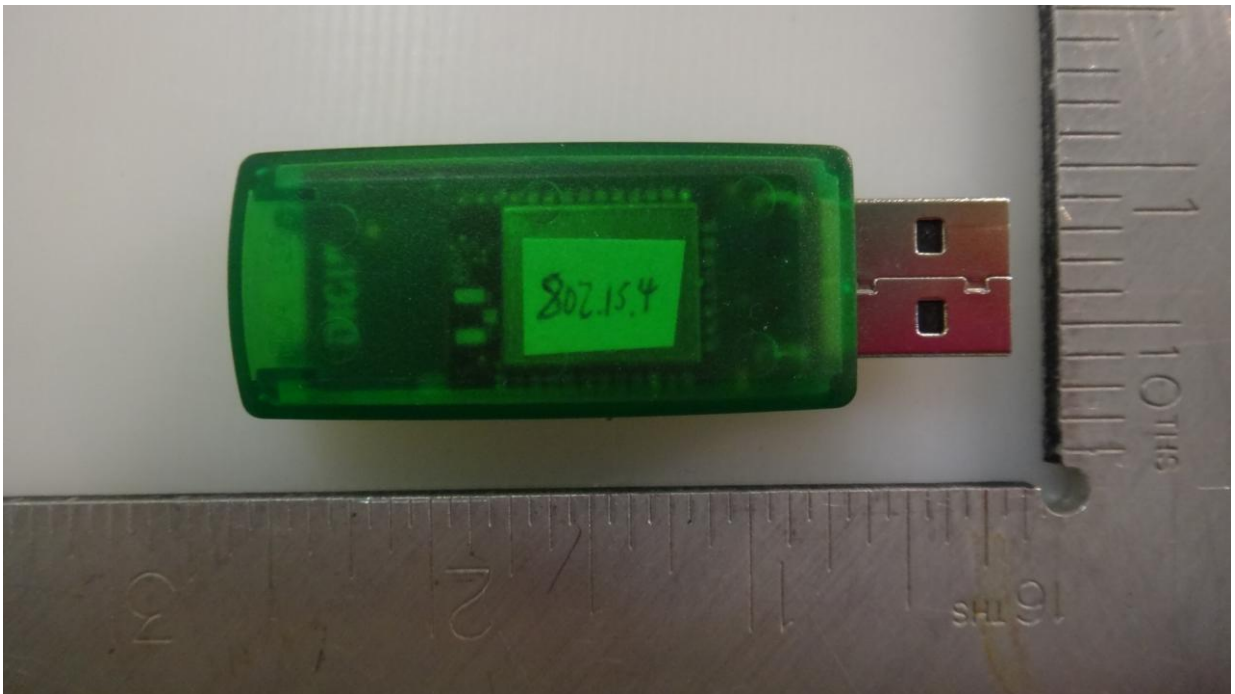
< D.U.T.'s rear view with 802.15.4 Encoded Radio >
