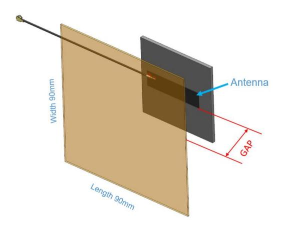
FIGURE 6.1.1 FOUR LOCATIONS WITH PARALLEL PLANE GROUND
