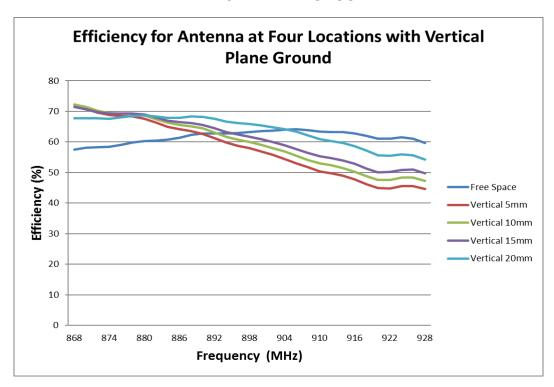
FIGURE 6.2.3 EFFICIENCY OF ANTENNA AT 868/915MHZ AT FOUR LOCATIONS WITH VERTICAL PLANE GROUND
