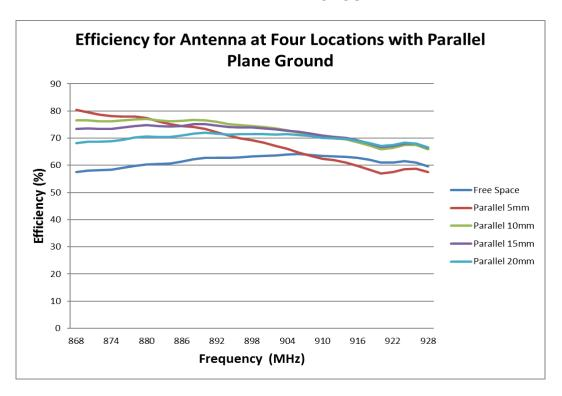
FIGURE 6.1.3 EFFICIENCY OF ANTENNA AT 868/915MHZ AT FOUR LOCATIONS WITH PARALLEL PLANE GROUND
