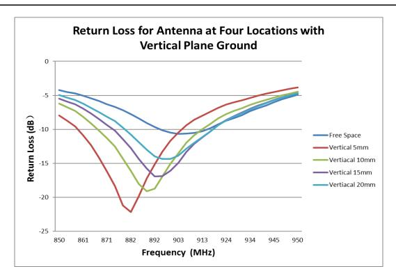
FIGURE 6.2.2 RETURN LOSS OF ANTENNA AT 868/915MHZ AT FOUR LOCATIONS WITH VERTICAL PLANE GROUND
