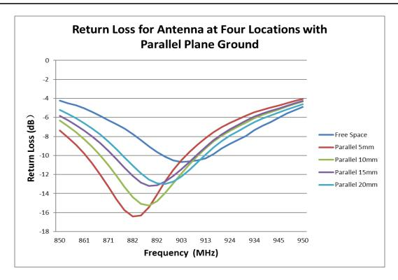
FIGURE 6.3.2 RETURN LOSS OF ANTENNA AT 868/915MHZ AT FOUR LOCATIONS WITH PARALLEL PLANE GROUND
