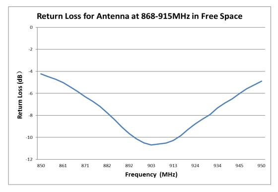
FIGURE 4.3.1 RETURN LOSS OF ANTENNA AT 868/915MHZ IN FREE SPACE
