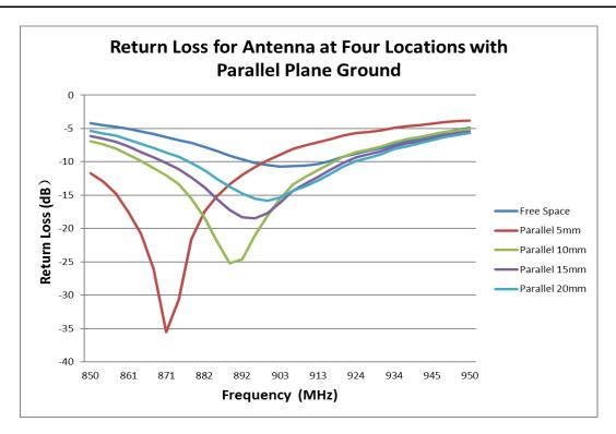
FIGURE 6.1.2 RETURN LOSS OF ANTENNA AT 868/915MHZ AT FOUR LOCATIONS WITH PARALLEL PLANE GROUND
