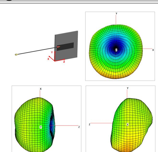
FIGURE 4.5.3 3D RADIATION PATTERN OF ANTENNA AT 868MHZ IN FREE SPACE
