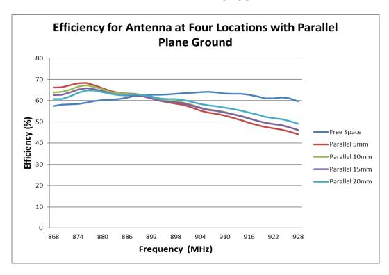
FIGURE 6.3.3 EFFICIENCY OF ANTENNA AT 868/915MHZ AT FOUR LOCATIONS WITH PARALLEL PLANE GROUND
