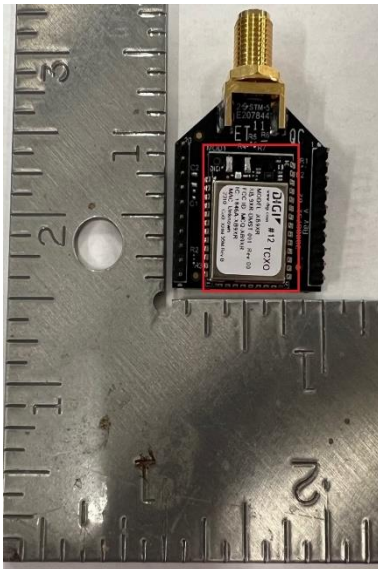
XBee XR 900 with RF-pad output on pin side of module carrier
