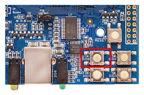
On the board you see **DIOO** written below **SW2**, to the left of the button. This represents the pin that the button is connected to.
