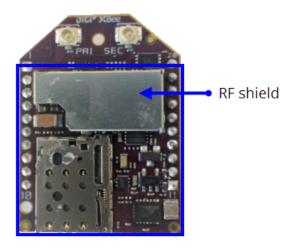
When attaching to the host PCB, tighten the mounting hardware until the gasket is compressed at least 25% and the heat sink is snug against the RF shield. Avoid overtightening. To prevent shorting, check that the surface of the heat sink does not directly contact any of the XBee device components.
