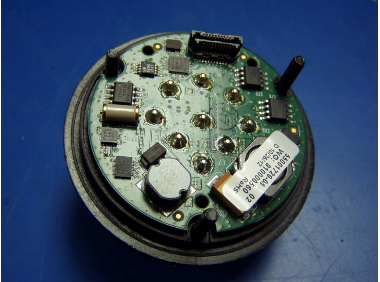
Assembly minus top, RF board, heatsink, cpu board, support ring
