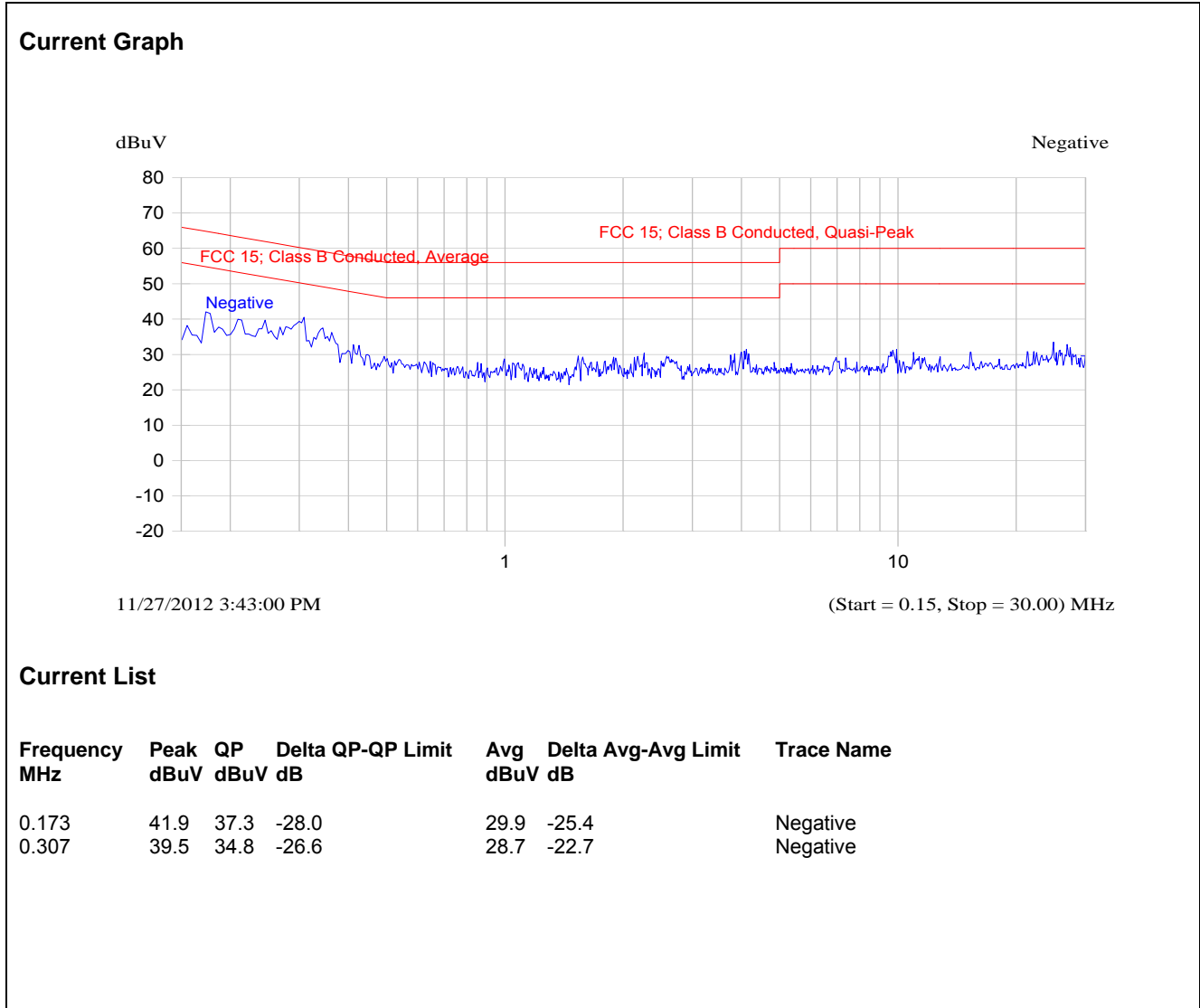
Plot 5.1.4.2. Power Line Conducted Emissions; Line Voltage: 3.6 V DC; Line Tested: Negative
