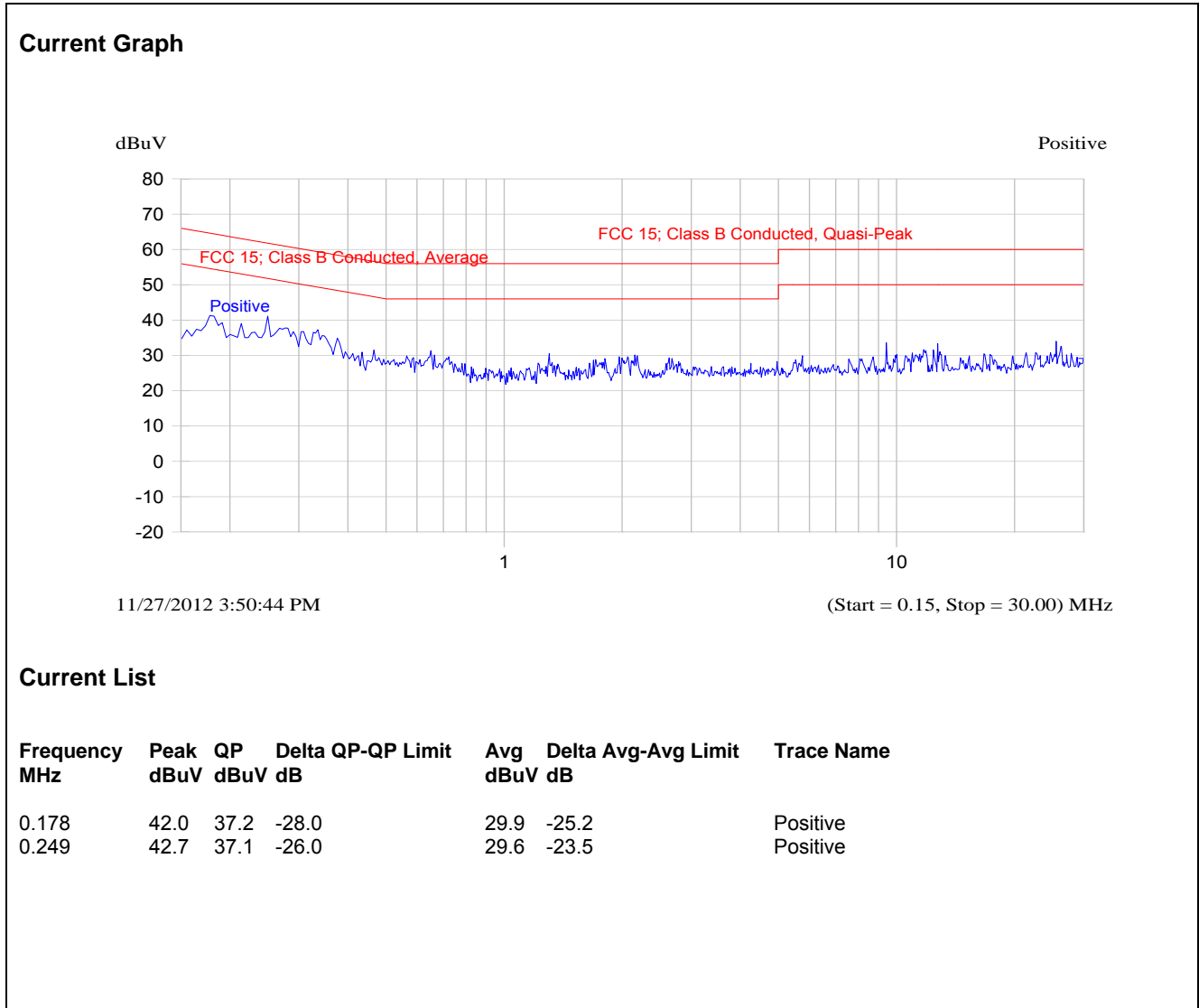
Plot 5.1.4.1. Power Line Conducted Emissions; Line Voltage: 3.6 V DC; Line Tested: Positive
