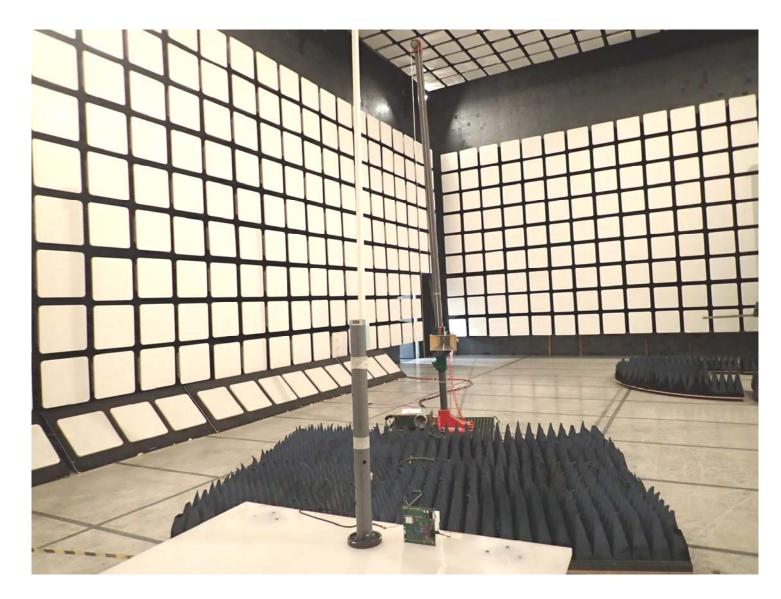
Radiated Emissions @ 3 m, Orthogonal Position 2 EUT with 15 dBi Omni-directional Antenna
