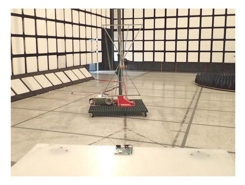
Radiated Emissions @ 3 m, Orthogonal Position 1 EUT with 0 dBi Integral Antenna
