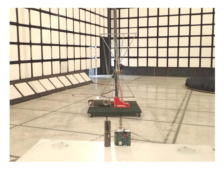
Radiated Emissions @ 3 m, Orthogonal Position 3 EUT with 2.1 dBi Dipole Antenna
