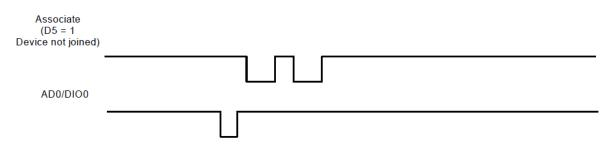
The following image illustrates the behavior pressing the button once on a remote device, causing a broadcast node identification transmission to be sent. All devices that receive this transmission blink their associate pin rapidly for one second if the associate LED functionality is enabled (**D5** = 1).
