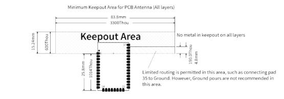
Recommended Keepout Area for PCB Antenna (All layers)
