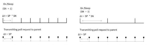
Setting SN > 1 allows the device to silently poll for data without asserting On/Sleep. If RF data is received when polling, On/Sleep will immediately assert.
