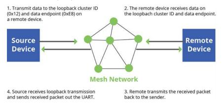
The configuration steps for sending data to the loopback cluster ID depend on what mode the device is in. For details on setting the mode, see AP (API Enable). The following sections list the steps based on the device's mode.
