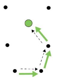
After obtaining a source route, the data collector sends a source routed transmission to the remote device.
