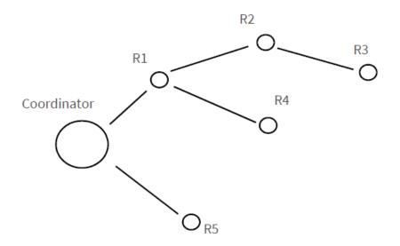
To send a source-routed packet to R3, the application sends a Create Source Route API frame (0x21) to the XBee, with a destination of R3, and 2 hops (R1 and R2). If the 64- bit address of R3 is 0x0013A200 404a1234 and the 16-bit addresses of R1, R2, and R3 are:
