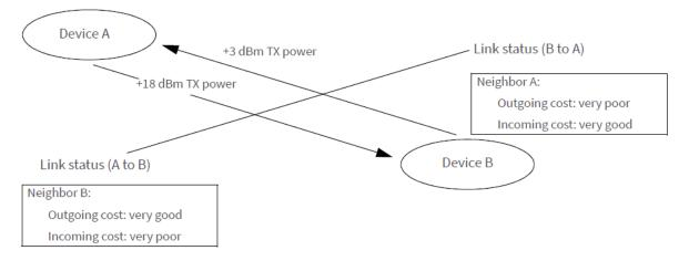
This mechanism enables devices A and B to recognize that the link is not reliable in both directions and select a different neighbor when establishing routes. Such links are called asymmetric links, meaning the link quality is not similar in both directions.
