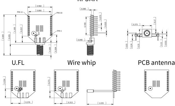
The drawings below show the XBee-PRO through-hole model.
