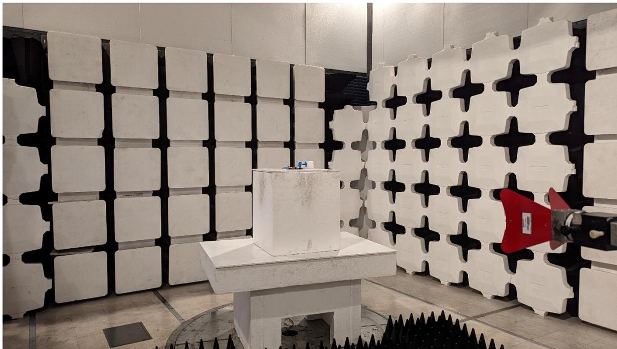
2.4GHz ANTX100P001B24553 Tx Spurious Emissions 1-18GHz
