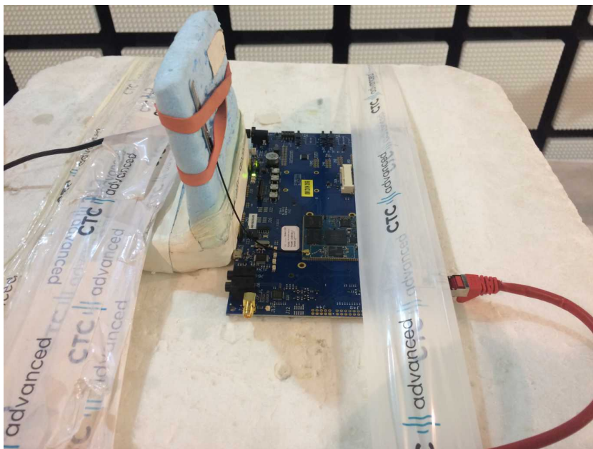
Photo 16: Fully anechoic chamber test setup (PCB Antenna, YAGEO ANTX100P001B24553)
