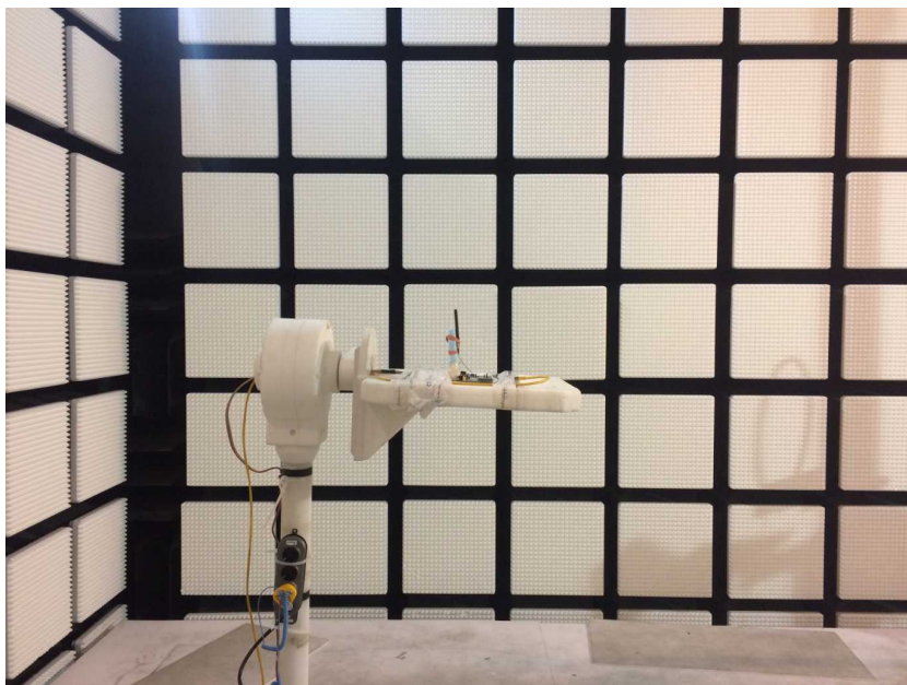
Photo 14: Fully anechoic chamber test setup (Dipole Antenna, TAOGLAS GW48.151)
