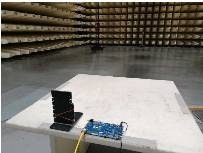
Photo 8: Semi anechoic chamber test setup (Dipole Antenna, Linx ANT-DB1-RAF-RPS)
