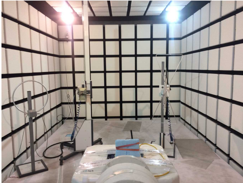
Photo 15: Fully anechoic chamber test setup (Dipole Antenna, TAOGLAS GW48.151)
