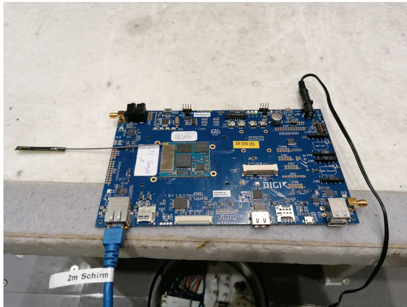
Photo 11: Semi anechoic chamber test setup (PCB Antenna, TAOGLAS FXP831.07.0100C)
