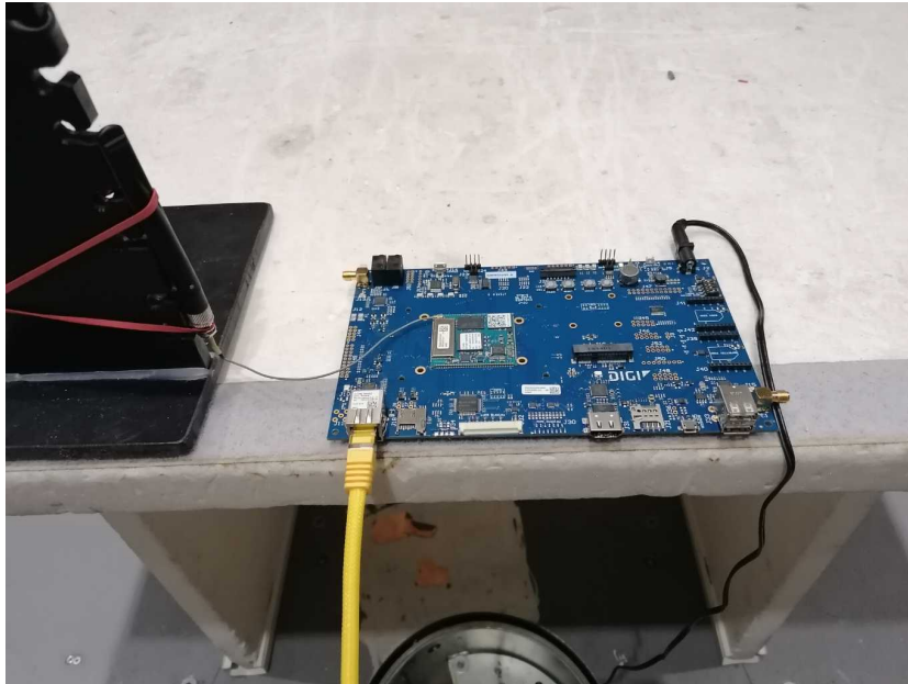
Photo 7: Semi anechoic chamber test setup (Dipole Antenna, Linx ANT-DB1-RAF-RPS)
