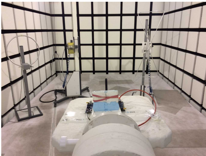
Photo 20 : Fully anechoic chamber test setup (Dipole Antenna, Linx ANT-DB1-RAF-RPS)
