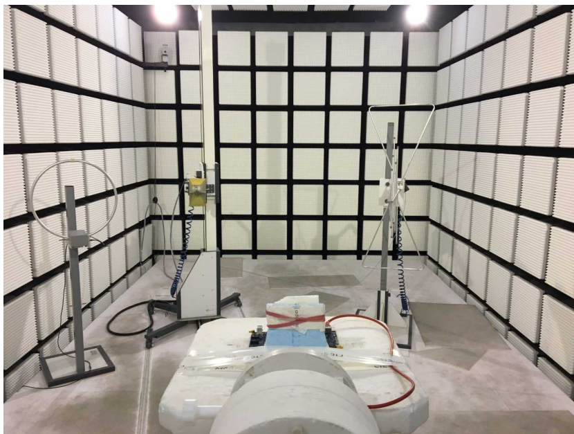
Photo 24: Fully anechoic chamber test setup (PCB Antenna, TAOGLAS FXP831.07.0100C)
