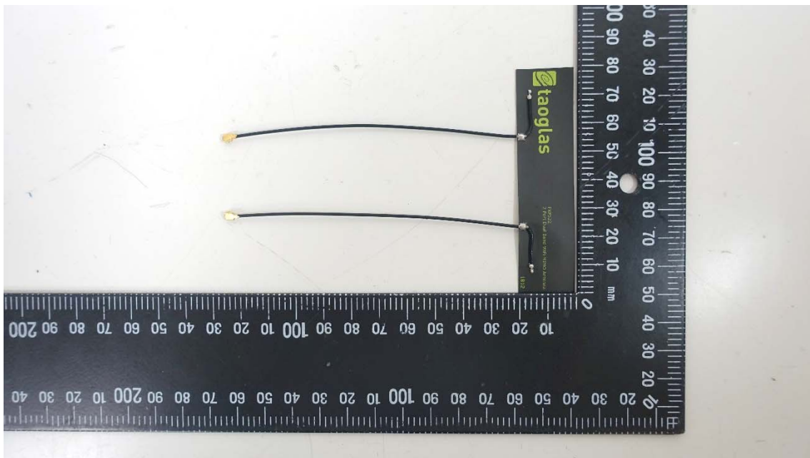
Antenna-4 (Model No.: FXP522.A.07.A.001)
