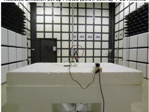
Radiated Emission Set up Photos (Below 30MHz) \*PCB Antenna
