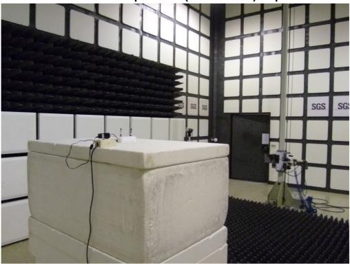
Radiated Emission Set up Photos (Above 1GHz) \*Dipole Antenna
