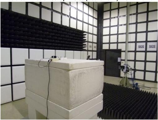
Radiated Emission Set up Photos (Above 1GHz) \*PCB Antenna
