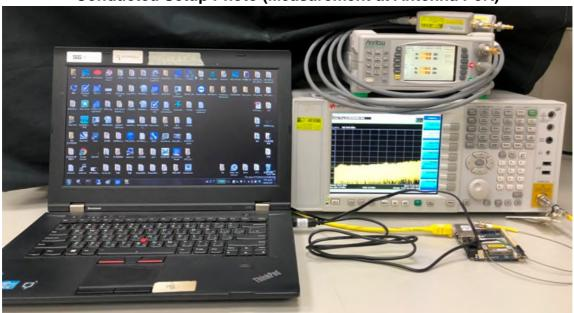
**Conducted Setup Photo (Measurement at Antenna Port)**
