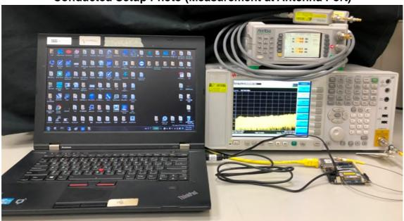
**Conducted Setup Photo (Measurement at Antenna Port)**
