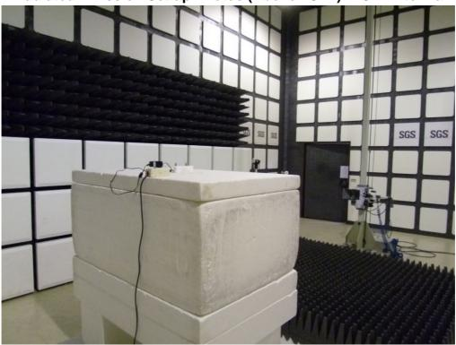
Radiated Emission Set up Photos (Above 1GHz) \*PCB Antenna
