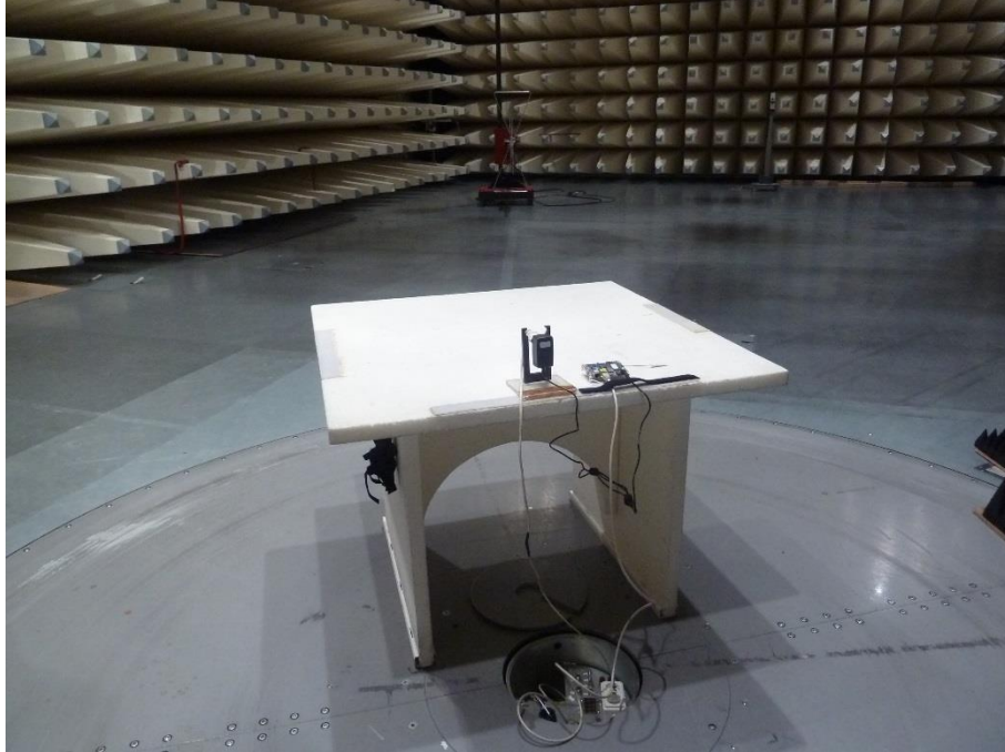
Photo 13: EUT with PCB antenna at the anechoic chamber
