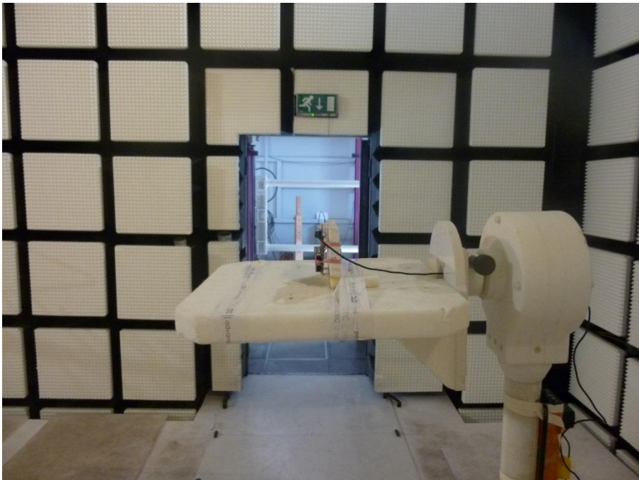
Photo 4: EUT with PCB antenna at the anechoic chamber
