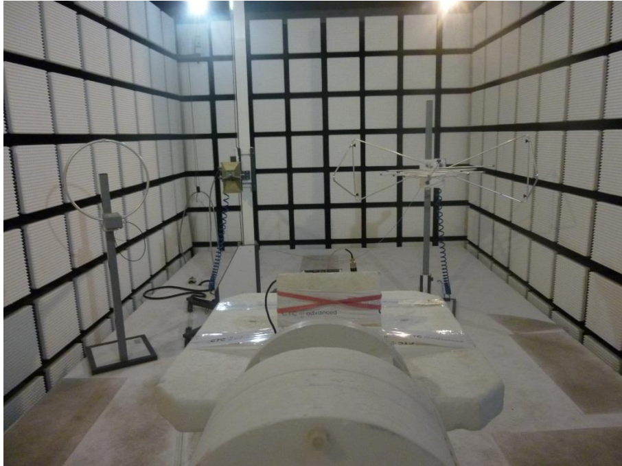
Photo 9: EUT with dipole antenna at the anechoic chamber
