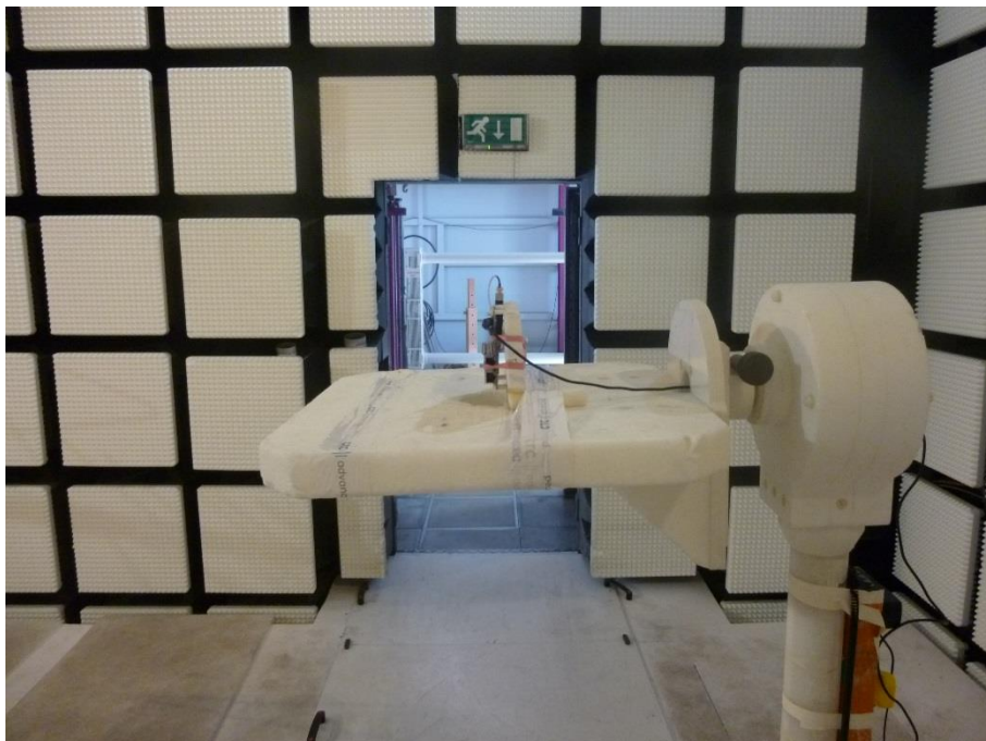
Photo 10: EUT with dipole antenna at the anechoic chamber
