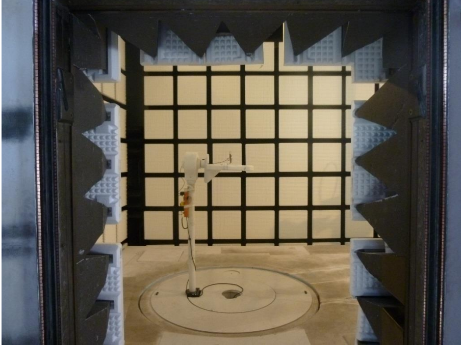
Photo 7: EUT with dipole antenna at the anechoic chamber
