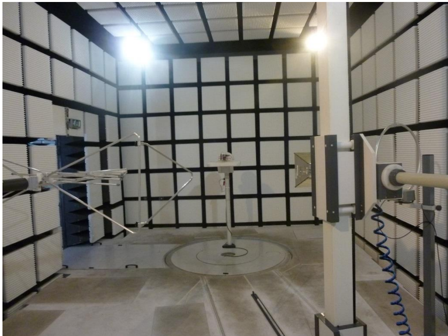
Photo 12: EUT with dipole antenna at the anechoic chamber
