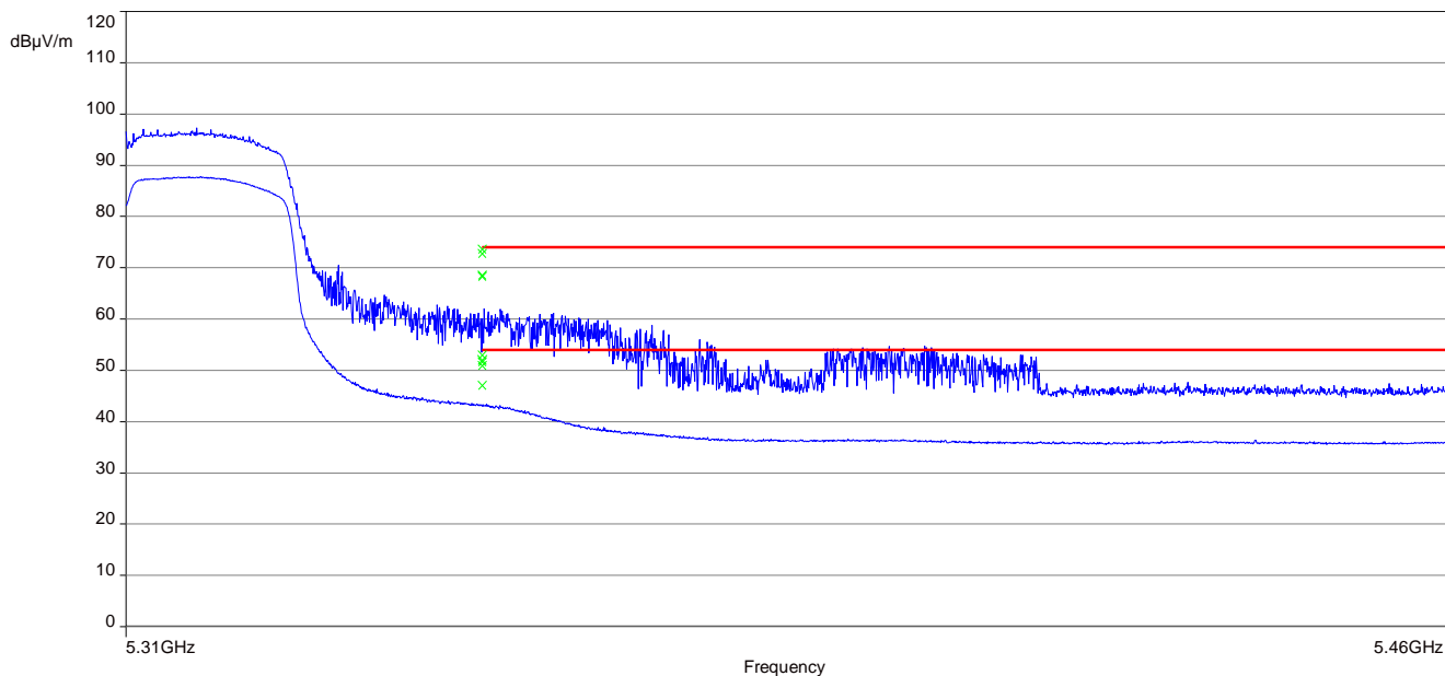
Plot 5: upper band edge; U-NII-2A; highest channel; 40 MHz channel bandwidth
