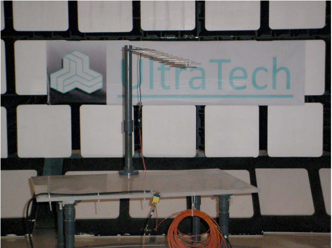
Radiated Emissions at 3 m EUT with 15.1 dBi Yagi Antenna (Orthogonal Position 3)
