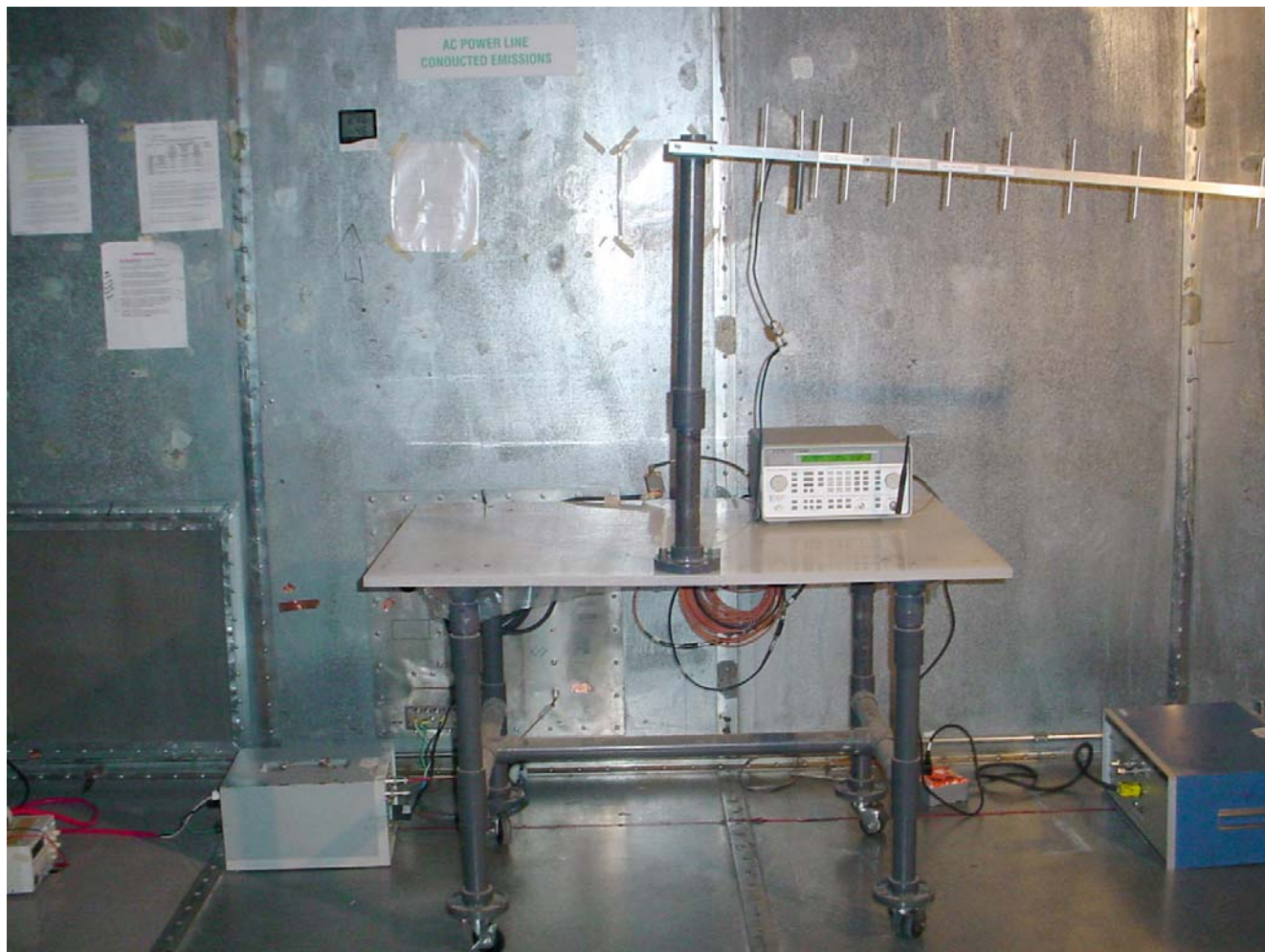
Power Line Conducted Emissions (Rx Mode)
