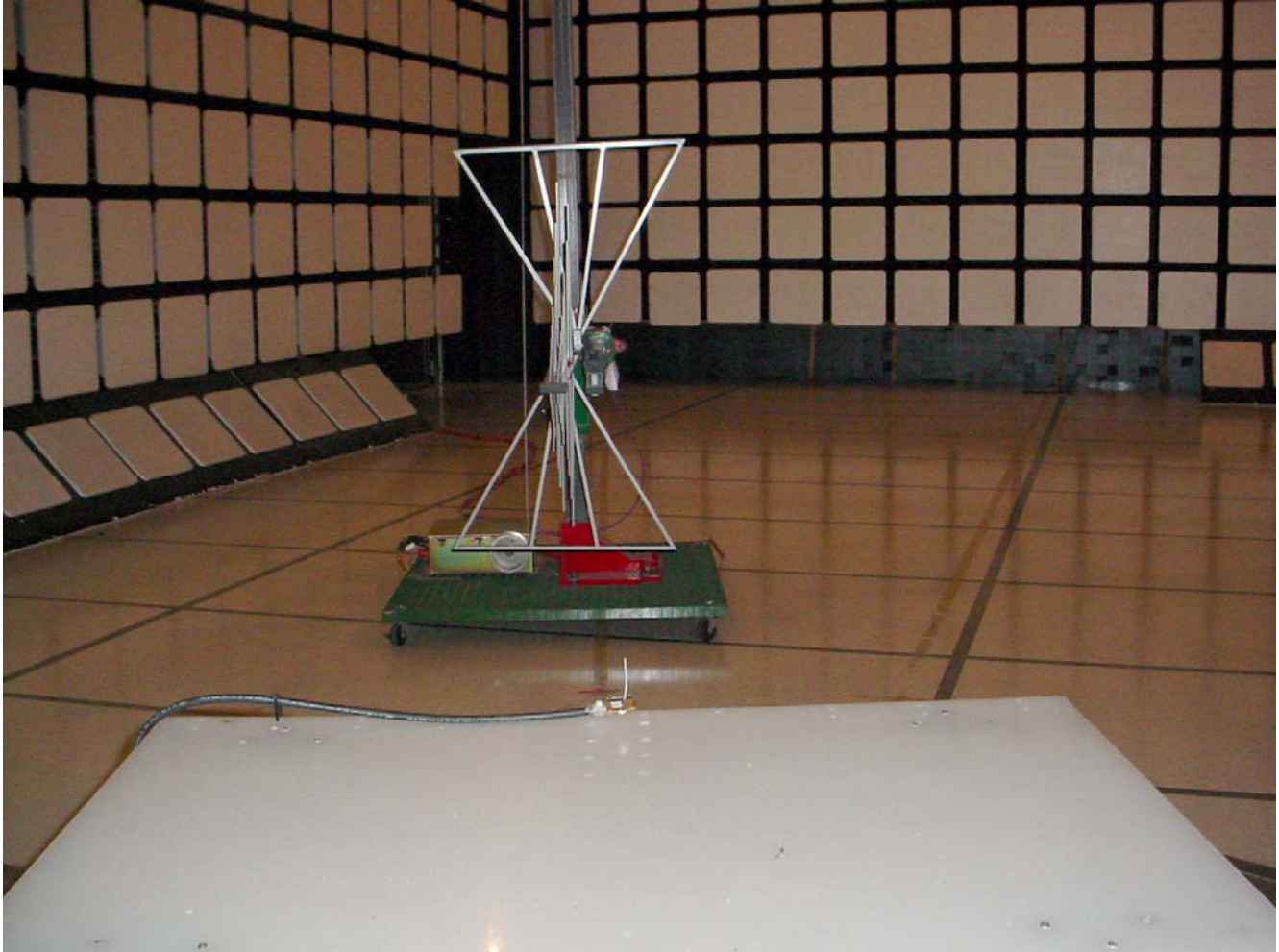
Radiated Emissions at 3 m EUT with 2.1 dBi Monopole Antenna (Orthogonal Position 1)
