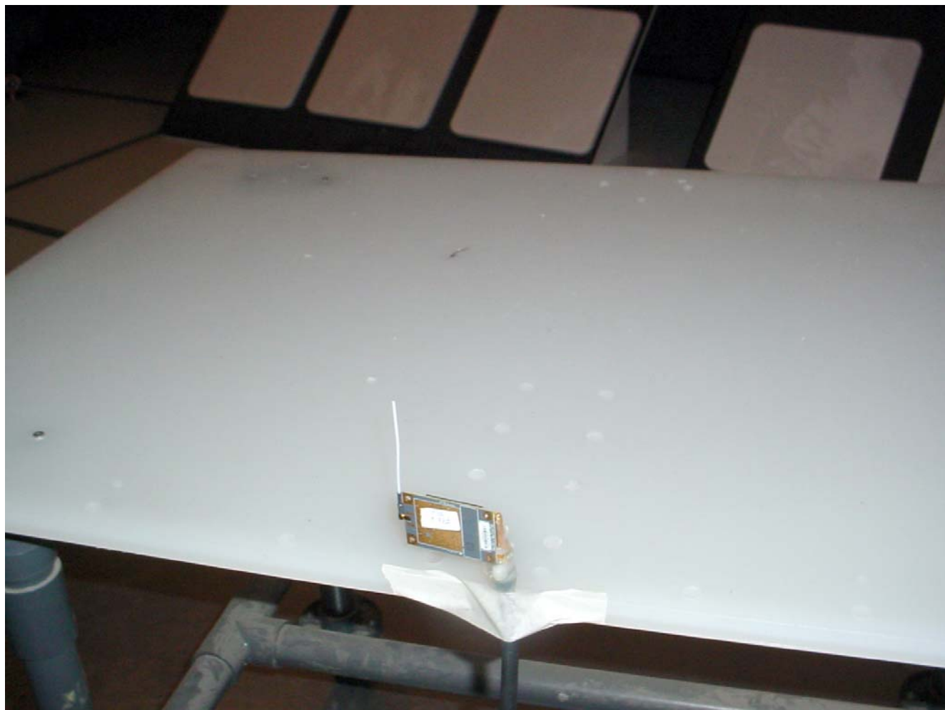
Radiated Emissions at 3 m EUT with 2.1 dBi Monopole Antenna (Orthogonal Position 2)
