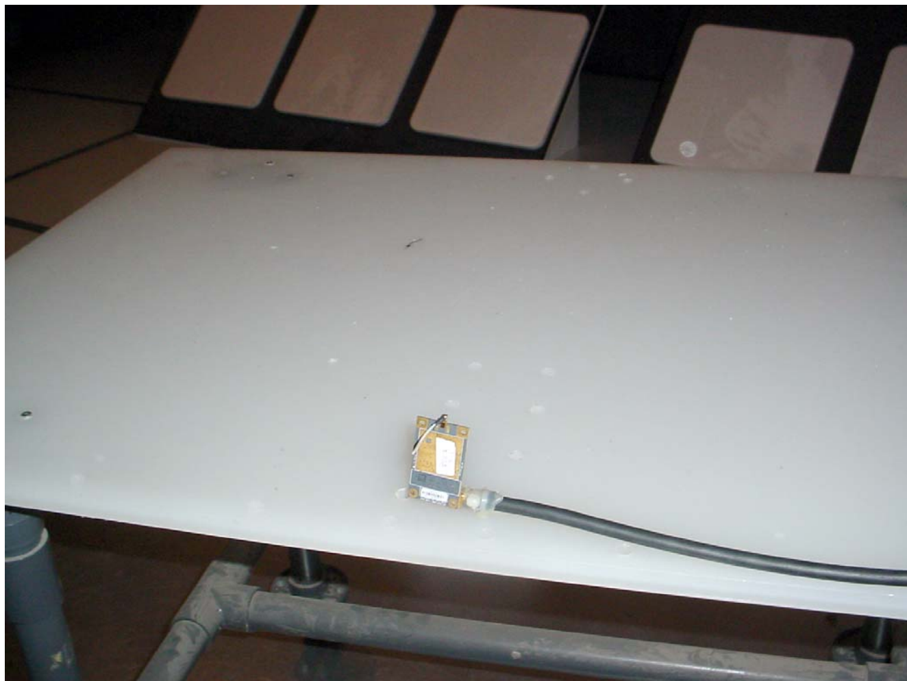
Radiated Emissions at 3 m EUT with 2.1 dBi Monopole Antenna (Orthogonal Position 3)
