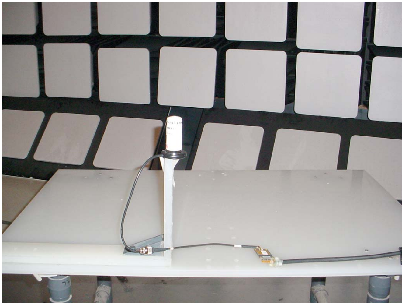
Radiated Emissions at 3 m EUT with 3.0 dBi Multi-path Antenna
