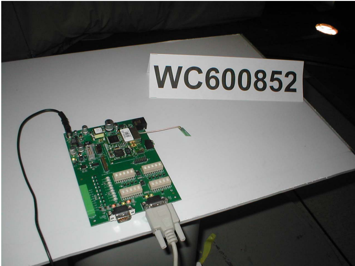
Test Set-up photo, radiated emissions
