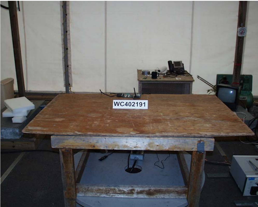
Test-setup photo(s): Radiated emission 30 MHz - 25000 MHz without 12" extension cable with antenna
