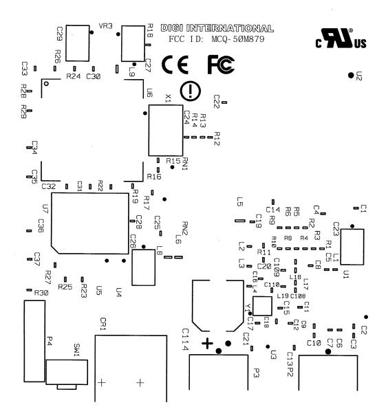
The FCC ID will be silkscreened on the device. Compliance statement will be placed on host device along with "Contains FCC ID: MCQ-50M879" and in manual. See other exhibits for details.
