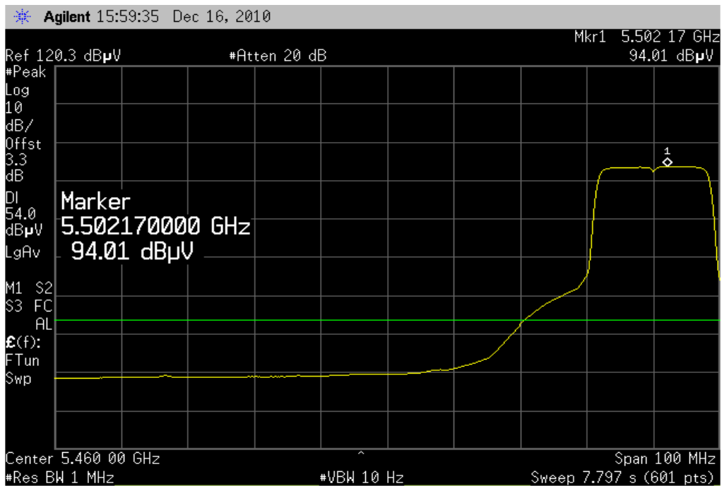
Plot 10: a – mode; lowest channel – 5500 MHz; power index 26; lower band edge; horizontal polarization
