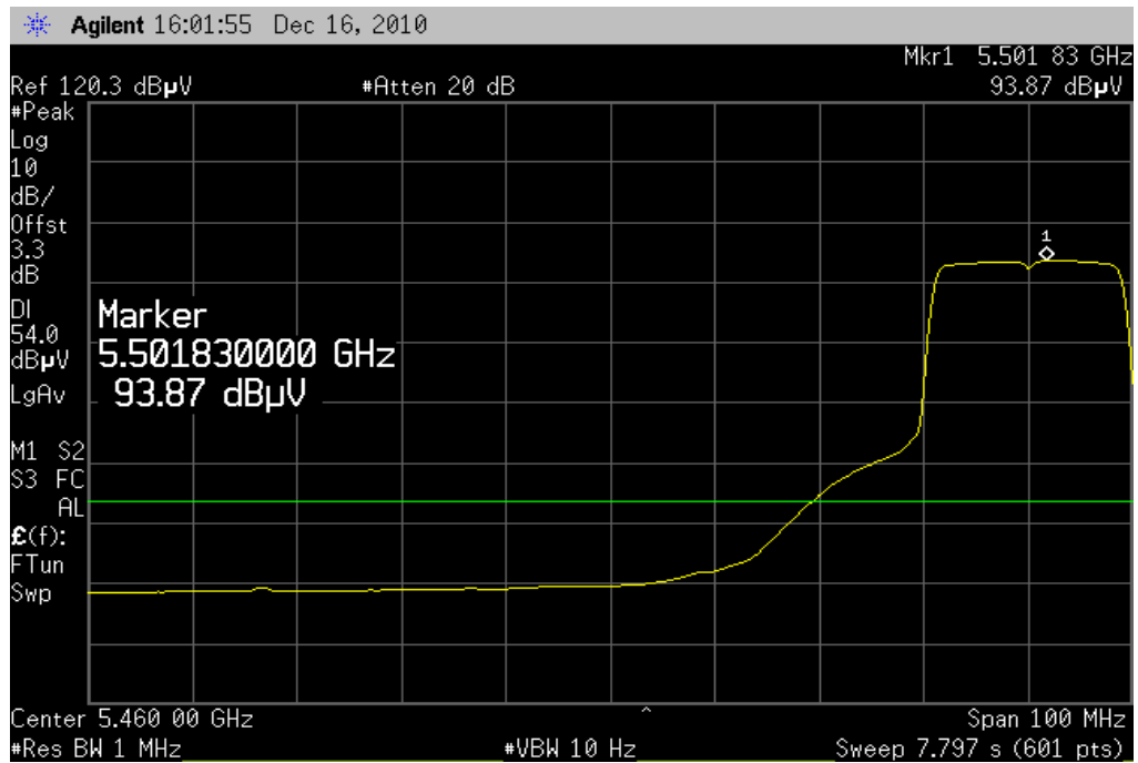
Plot 12: n – mode; lowest channel – 5500 MHz; power index 26; lower band edge; horizontal polarization
