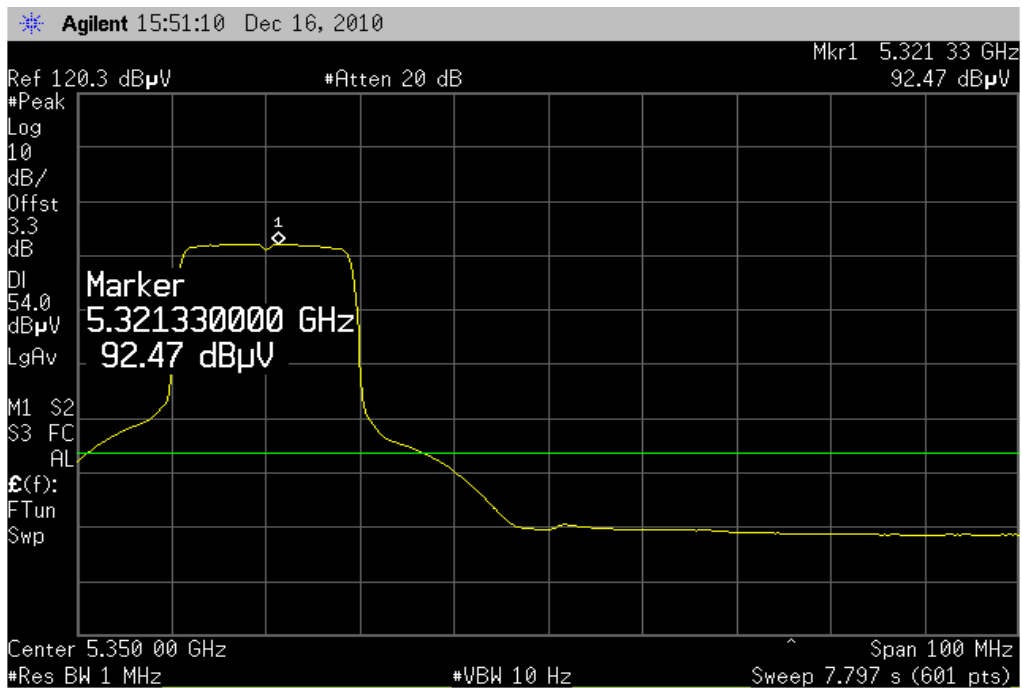
Plot 8: n – mode; highest channel – 5320 MHz; power index 21; higher band edge; horizontal polarization
