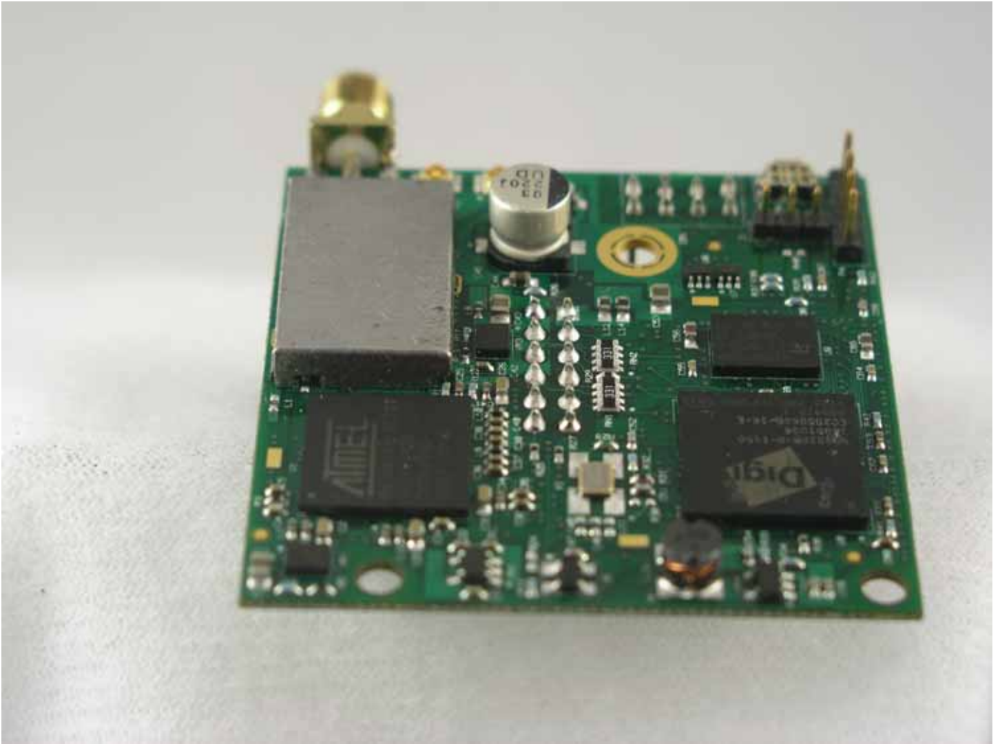
Digi WiEM 9210 Internal Photos – Shielding Details Left
