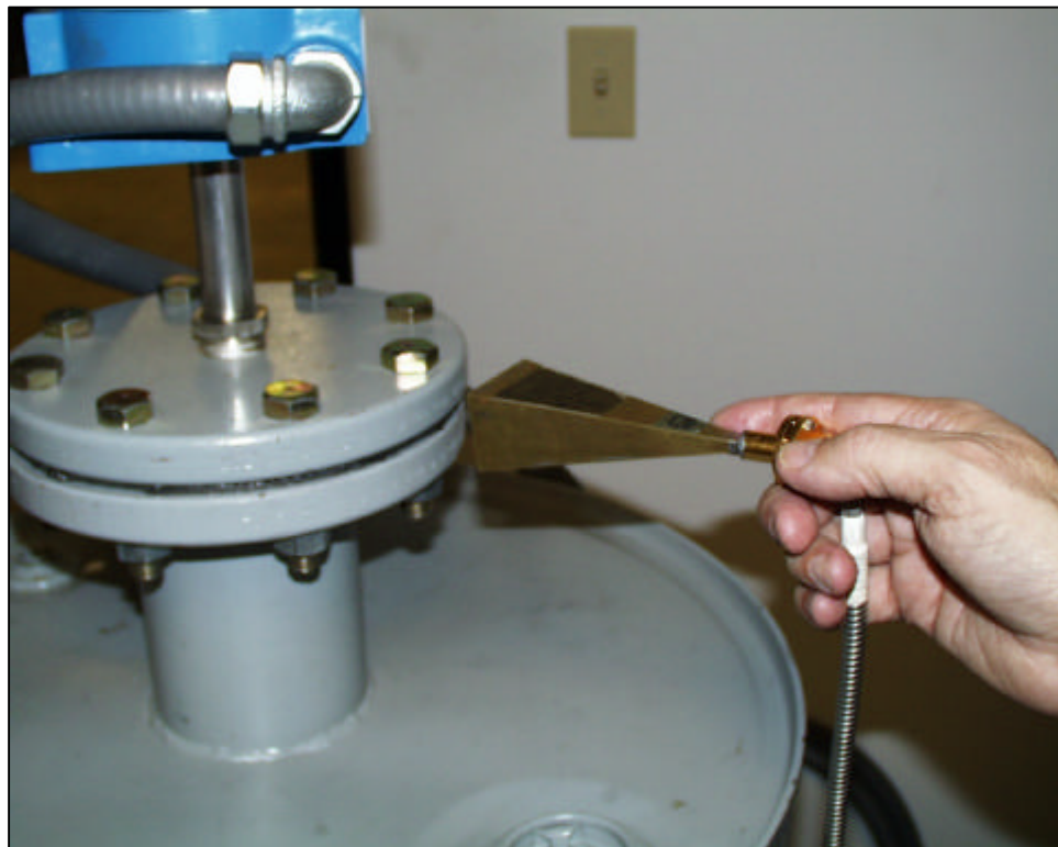
40 to 60 GHz Investigation of Possible Emissions From The Flange
