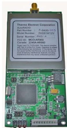
Figure 1. A Photograph of the modular transceiver
