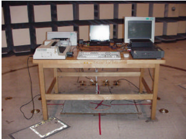
ThinkPad T30 (M/T 2366) Radiated measurement setup photo Front view
