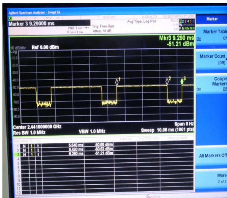
Time-domain plot for Bluetooth transmission signal
