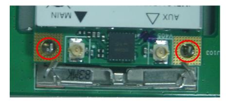
3. Assemble the Main and Aux antenna cable . Take the antenna cable from host device and link the connector with the connector on device .Press and make sure connection ok .
