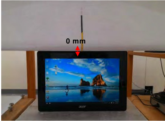
Fig.3 EUT Top side to flat phantom
