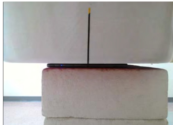
Fig.4 EUT Back side to flat phantom
