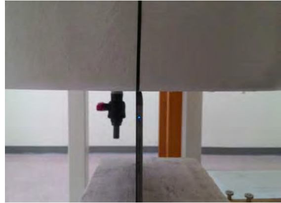
Fig.3 EUT Top side to flat phantom
