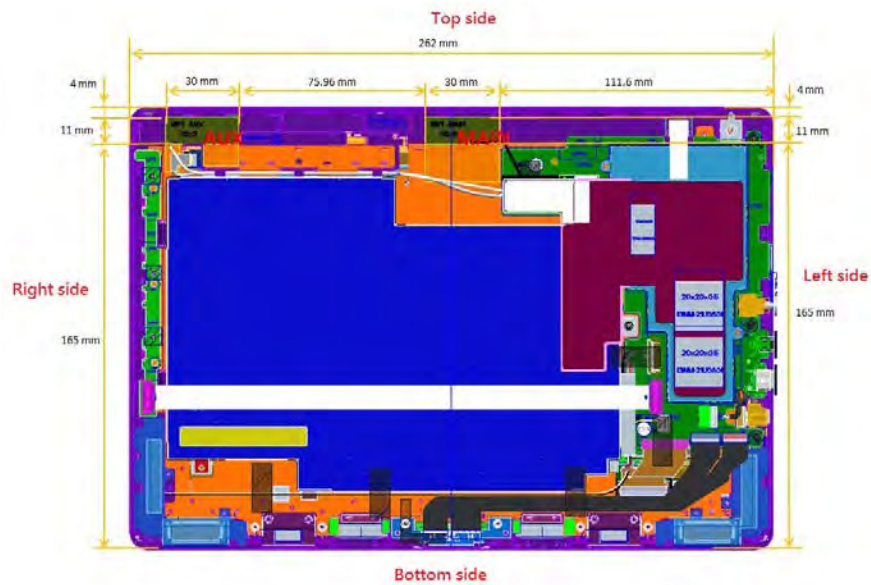
Fig.8 Antenna position of EUT (Back view)
