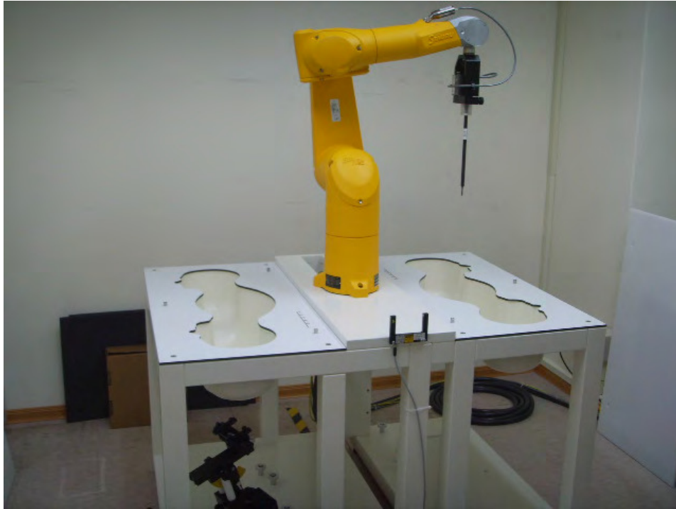
Fig.1 Photograph of the SAR measurement system
